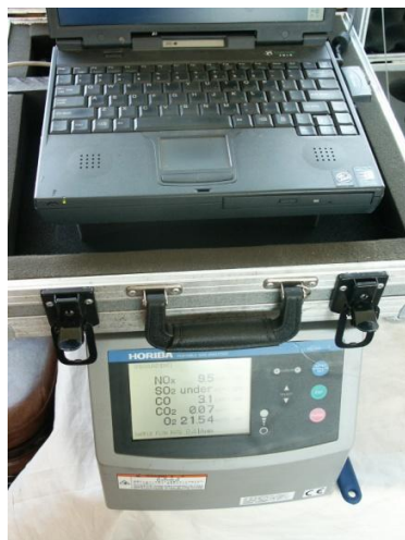
Figure A-3 Setup Showing Gas Analyzer with Computer for Continuous Data Logging
