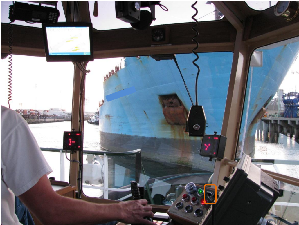
Figure 2-7 Wheelhouse on the Hybrid Tug shows Wheelhouse Switch in Orange Rectangle
