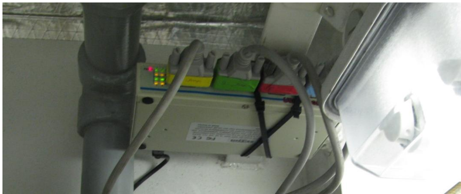
Figure 2-5 USB2-4COM-M - Receives serial signals from four engines and transmits them through one USB port to the data-logger
