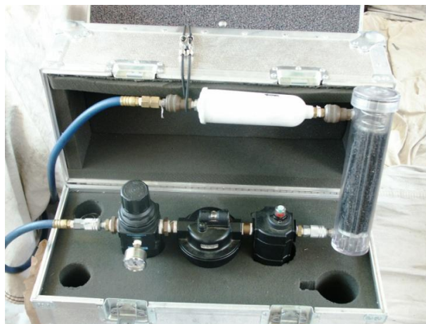
Figure A-2 Field Processing Unit for Purifying Dilution Air in Carrying Case
