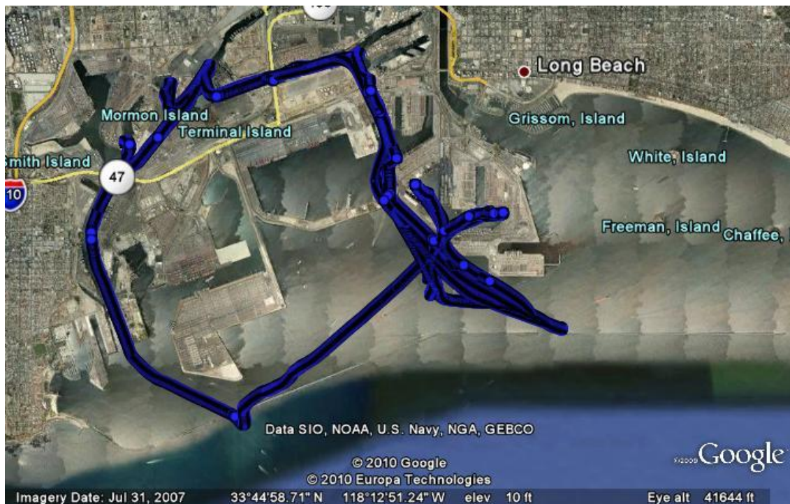
Figure 3-3 GPS data of a typical day for the Conventional Tug Note: Trace made by the blue dots indicates the route taken by the tug
