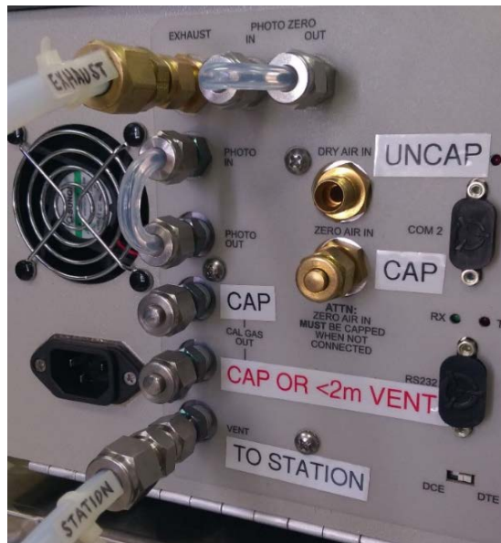
Figure 1: Example tubing configuration for presentation through-the-probe using a length of 3/8” outside diameter (OD) tubing. In this example, venting of bypass flow will be accomplished at the connection to the station’s sample probe, so the “Vent” port is left capped.
