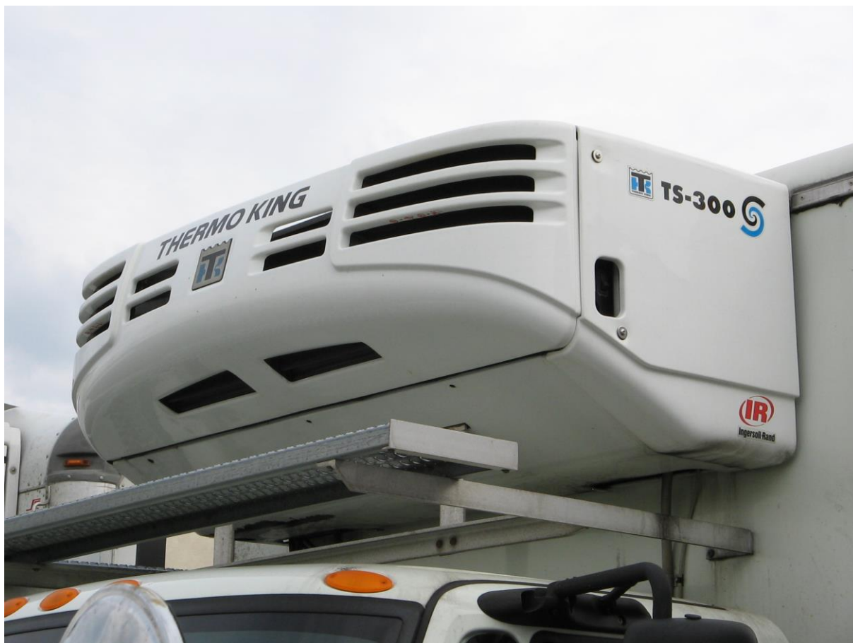
Figure 3-4. TRU unit installed on a Bobtail truck.
