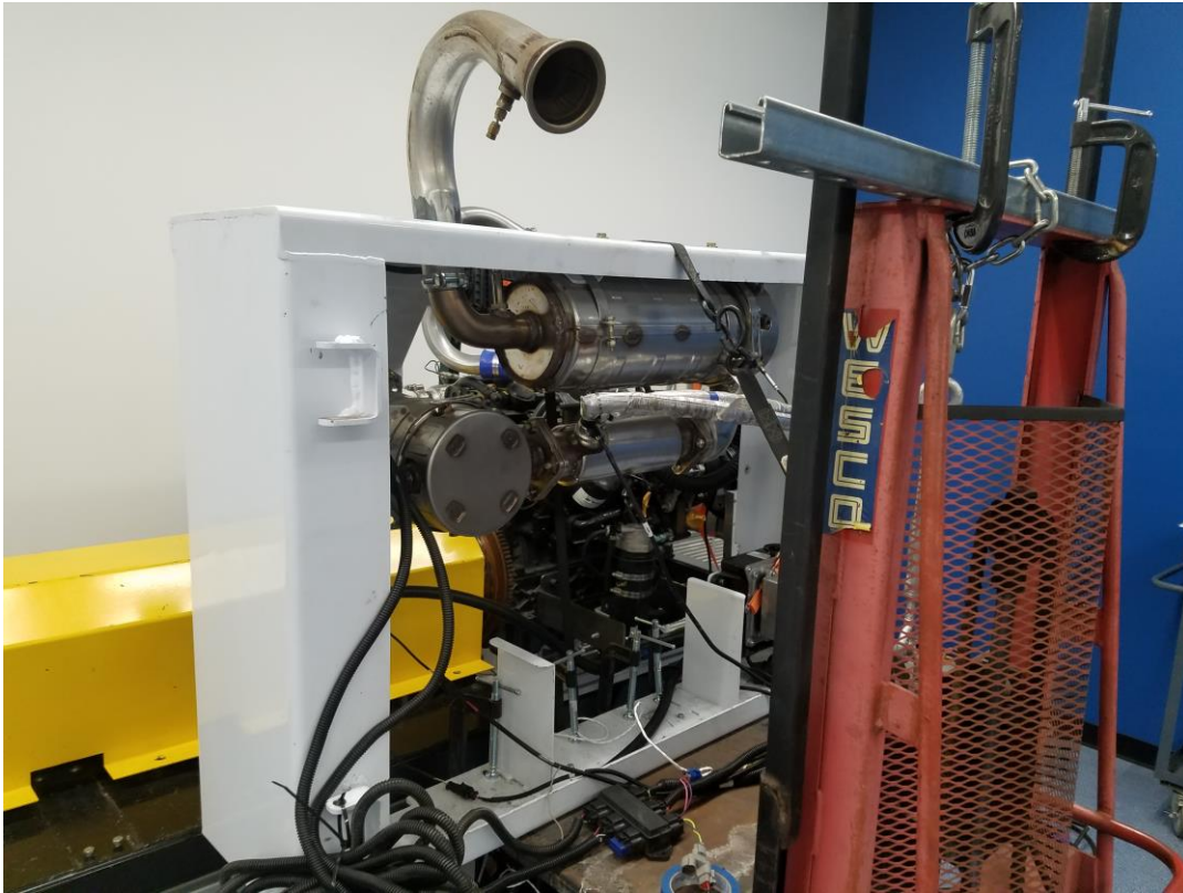
Figure 4-4. Skid Steer Engine on the Engine Dynamometer with the SCRT
