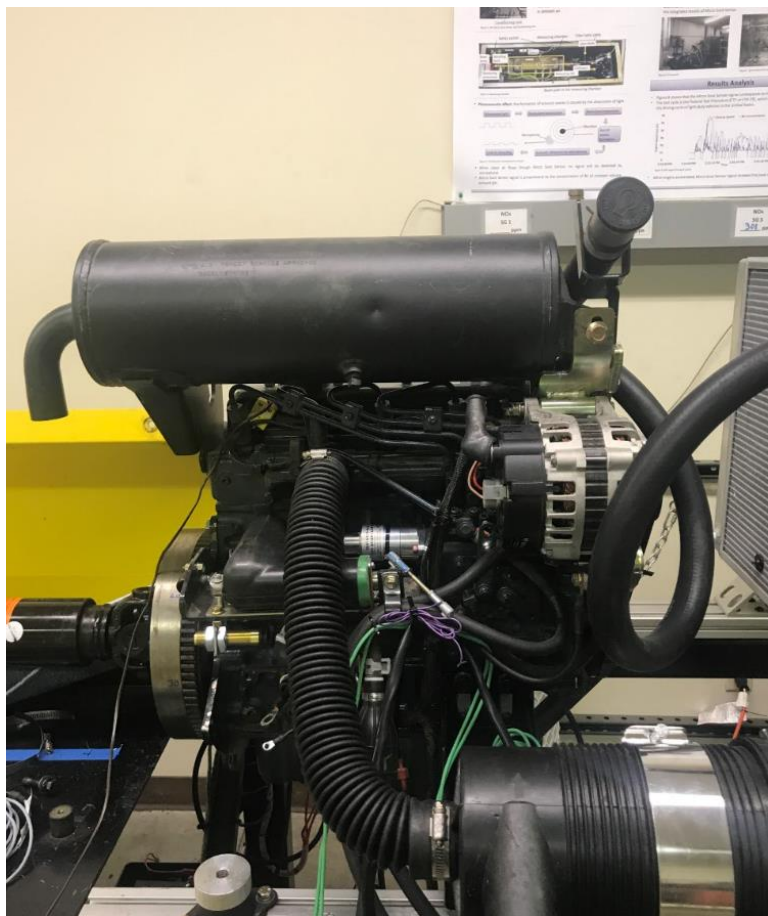
Figure 4-3. Mini-Excavator Engine on the Engine Dynamometer with the DPF
