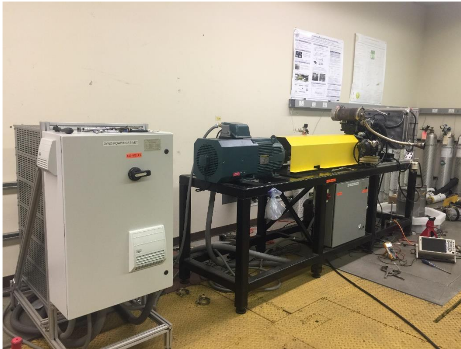
Figure 4-5. Engine Dynamometer used for Testing
