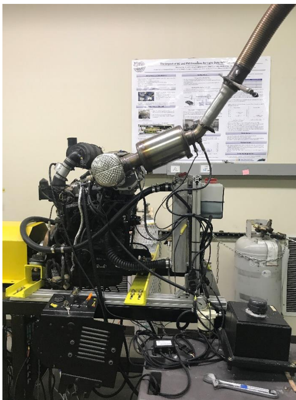
Figure 4-2. Ride Mover Engine on the Engine Dynamometer with the SCR
