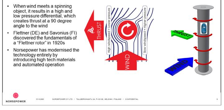
Rotor Sail is the most efficient mechanical sail in the world – it's physics are based on a pressure difference caused by the Magnus effect.
