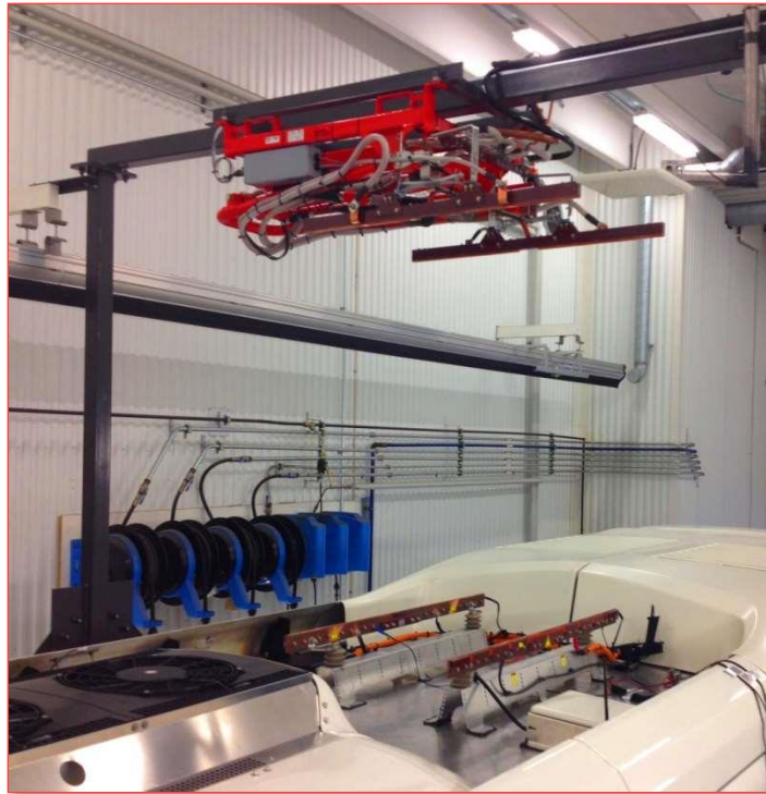
Figure 4-2. Inverted Pantograph and Charge Rails
