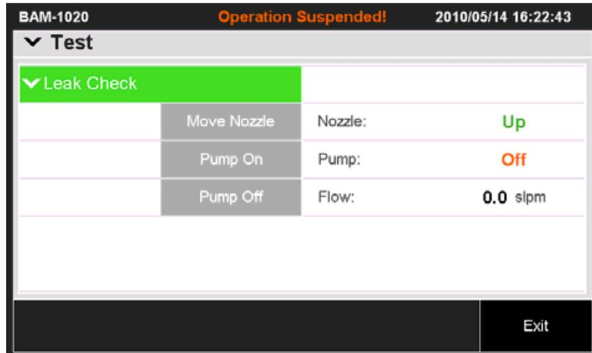
Figure AR-20. AM 1020 Touch Screen Leak Check Menu
