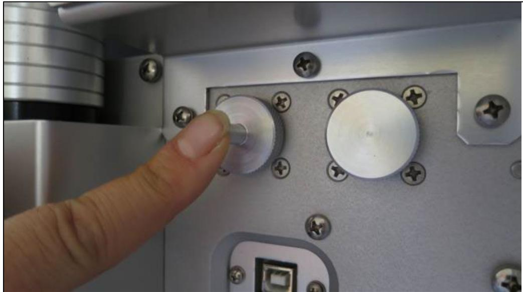
Figure AR-31. Met One E-BAM Plus Covering of Sheath Air Pre-Filter Inlet
