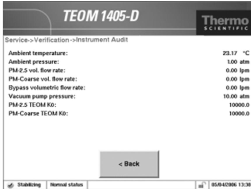
Figure AR-10. TEOM 1405-D Dichotomous Ambient Instrument Audit Screen.
