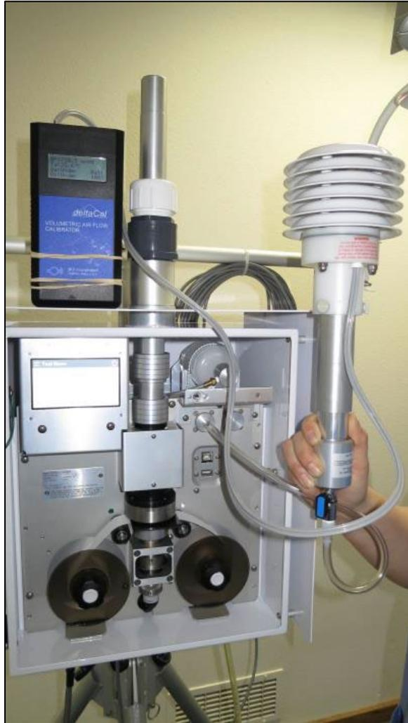
Figure AR-34. Met One E-BAM Plus Installation of Flow Audit Adapter and Audit Flow Standard
