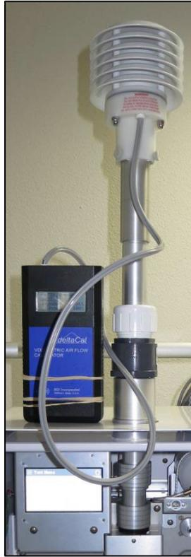
Figure AR-36. Met One E-BAM Plus Installation of Audit Flow Standard on Main Sample Inlet
