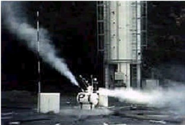
Excessive Tank Pressure (Blocking all safety valves)
