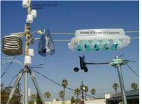
Initial results from laboratory and field evaluations of the passive samplers showed that several passive samplers demonstrated good precision. This was the case for nitrogen dioxide ( $NO_2$ ), nitrogen oxides ( $NO_2$ ), sulfur dioxide ( $SO_2$ ), formaldehyde, and acetaldehyde. However, results for other air toxics are still in the process of being evaluated. Lab and field set ups for testing the passive monitors are shown in the photographs on the right
