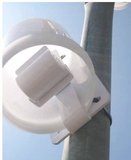
Ogawa passive samplers for NO x and SO 2 (thumb size in cup shield)
