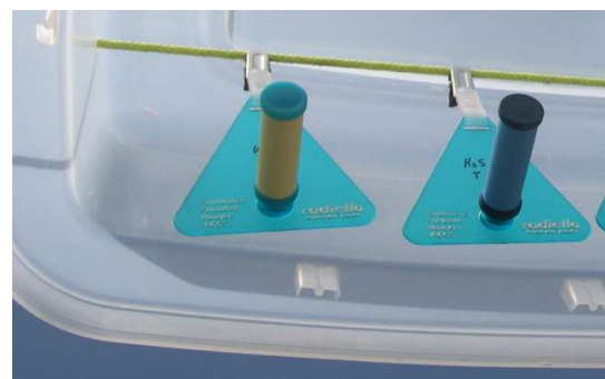
Radiello passive samplers for VOC, aldehydes and H 2 S (size of a roll of pennies)
