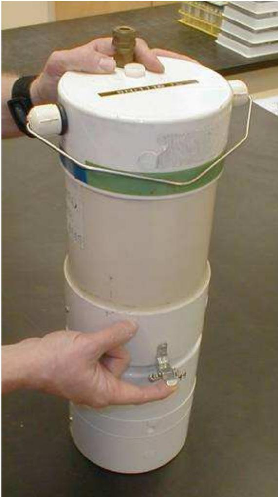
AirMetric Minivol Aerosol Sampler
