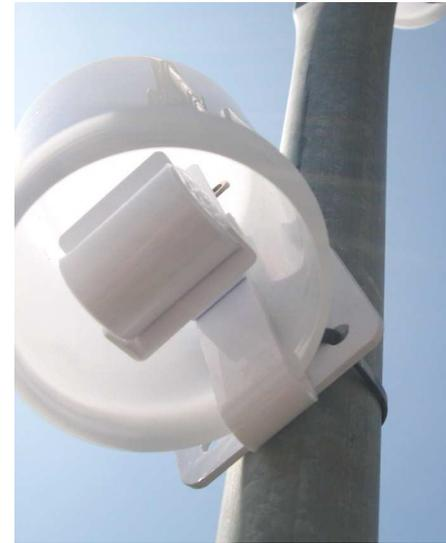
Ogawa passive samplers for NO<sub>x</sub> and SO<sub>2</sub>
