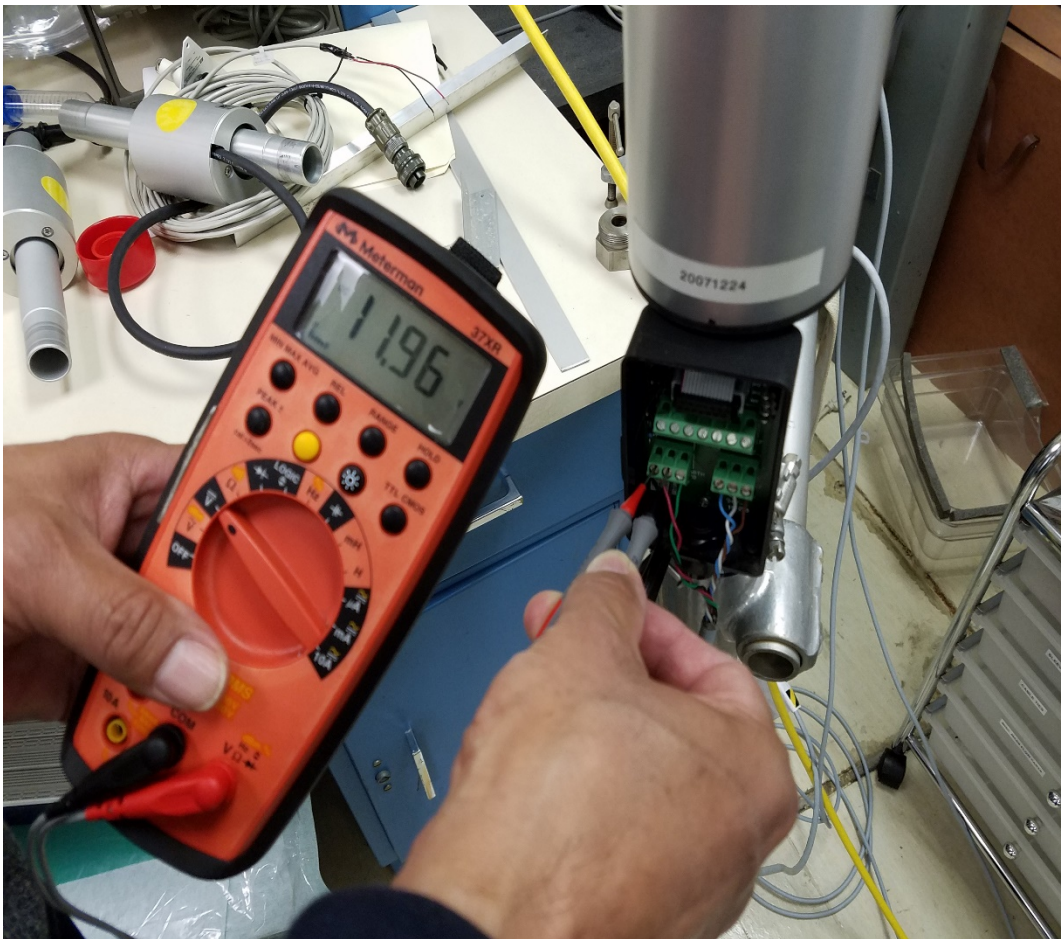
Figure 5: Checking 3D Sonic Input Voltage
