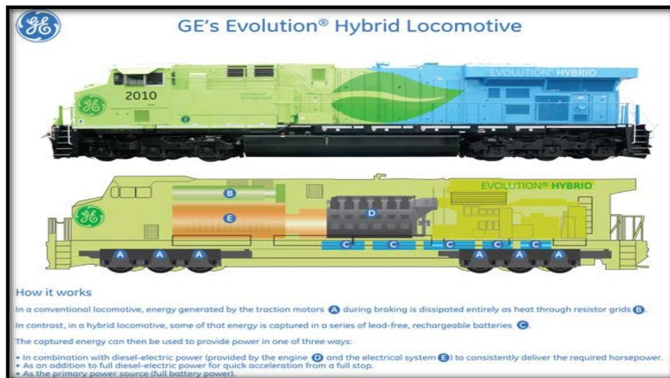
**Figure V-5: Picture of GE Evolution Battery-Hybrid Line Haul Locomotive**
