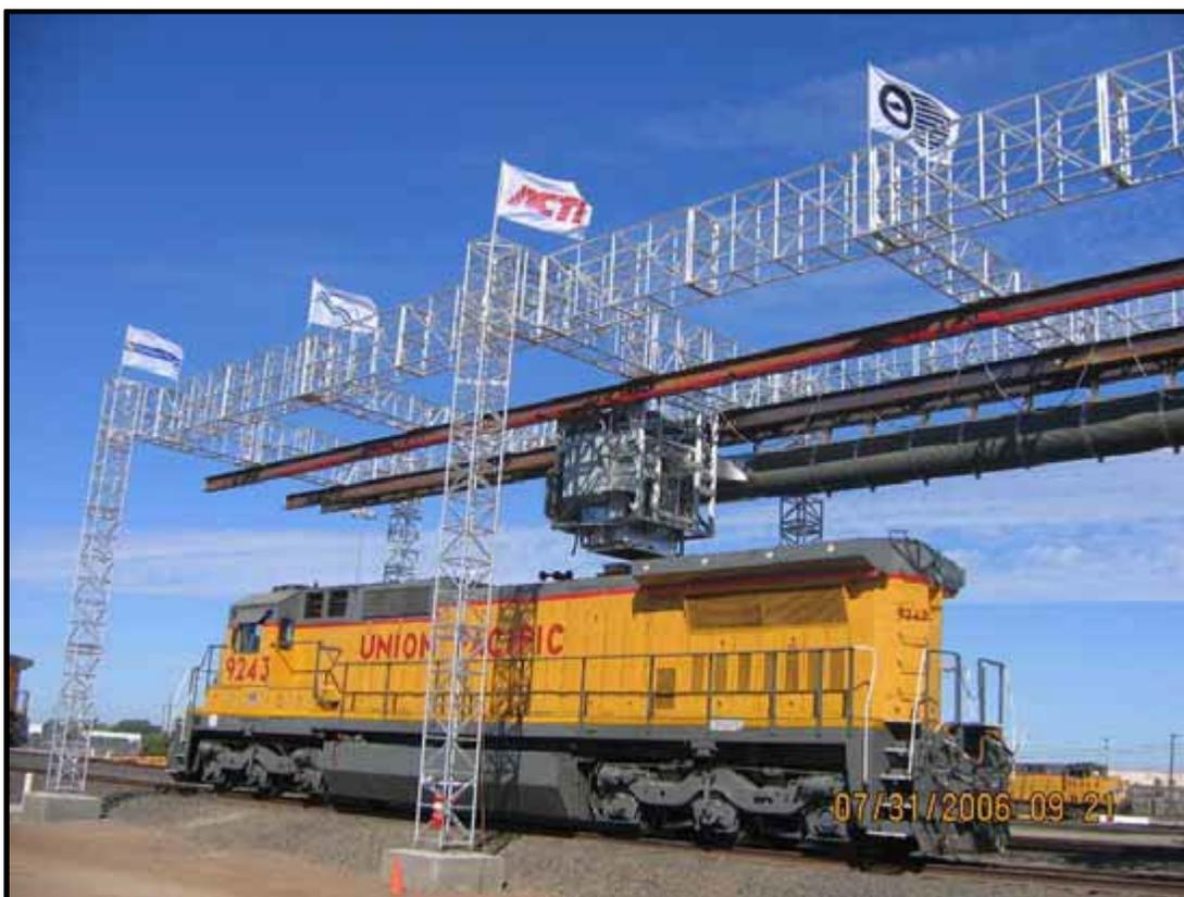
**Figure IX-1: Advanced Locomotive Emission Control System**
