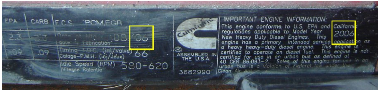
The Cummins ECL is typically on top of the engine, drivers' side. The image is of a 2007 vehicle model year. Note that the engine model year is 2006 and was compliant thru 2012. Most engines fall behind the truck model by one year.
