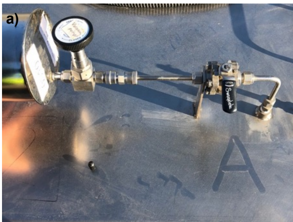
Figure 3.10 Gas Sample Collection
