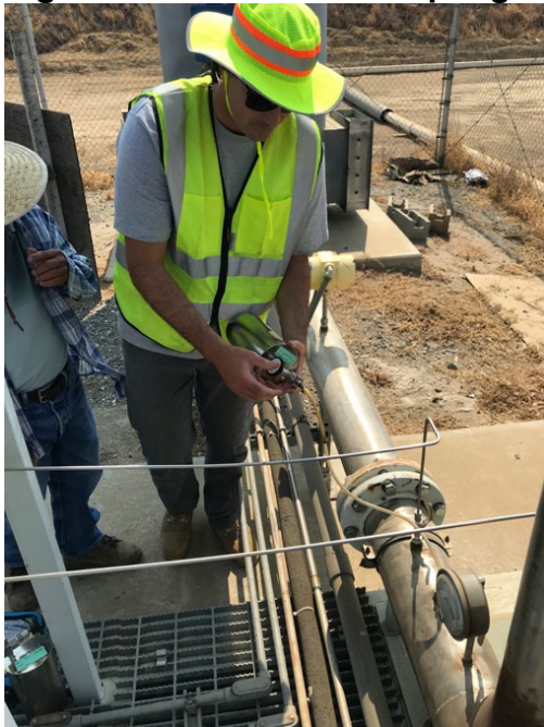
Figure 3.11 Raw Gas Sampling
