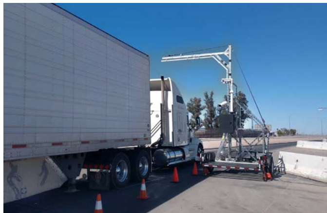
Heavy-duty vehicle driving through a PEAQs roadside unit
