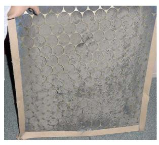
Dirty air filters can reduce airflow.
