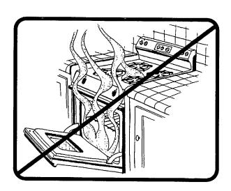
O Do not heat rooms or houses with kerosene- or gasfired space heaters. California law prohibits the advertising and sale of such unvented combustion space heaters for residential use, and State building standards require combustion heating systems to be vented directly to the outside.
