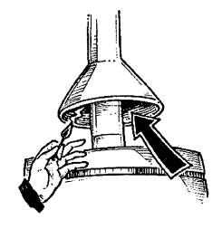
o Spillage indicators are heat-sensitive dots on a small card that will change color if they detect any significant spillage of hot combustion gases. They cost about \$3. Consider attaching them to gas furnaces and water heaters. Check them weekly and replace them annually. Also check near the flue for extensive rust or soot as an indicator of spillage.
