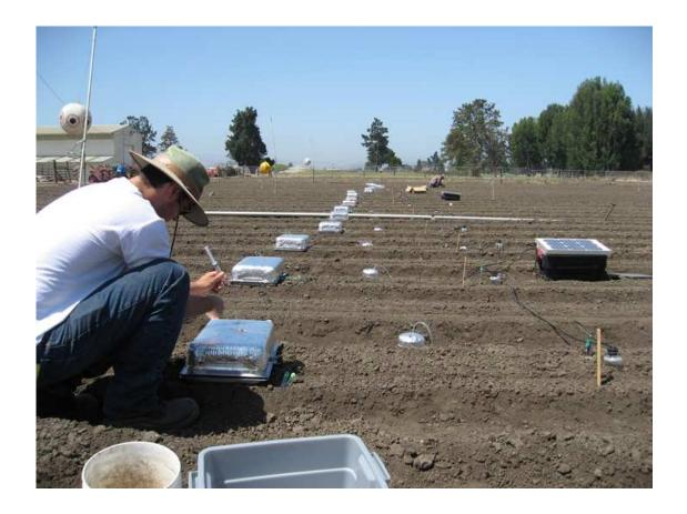
Static chamber technique will be used to collect air samples and measure  $\rm N_2O$  flux from dairy forage fields
