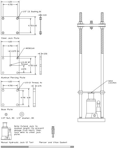
1/2-13 Steel Retaining Rod - 30" Length, 4X
