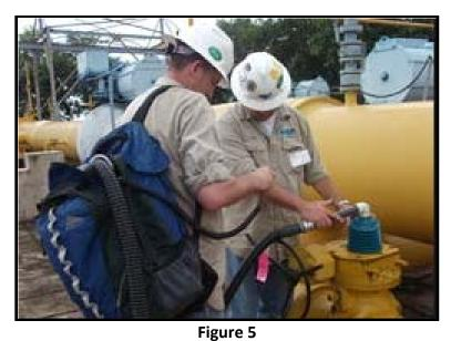
Hi Flow measurement of a leak interface from a valve at a natural gas well pad.
