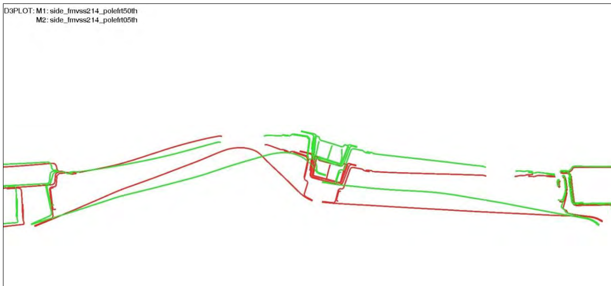
Figure 4.5.4.3.1.a: 5 th percentile female vs. 50 th percentile male front door intrusion comparison
