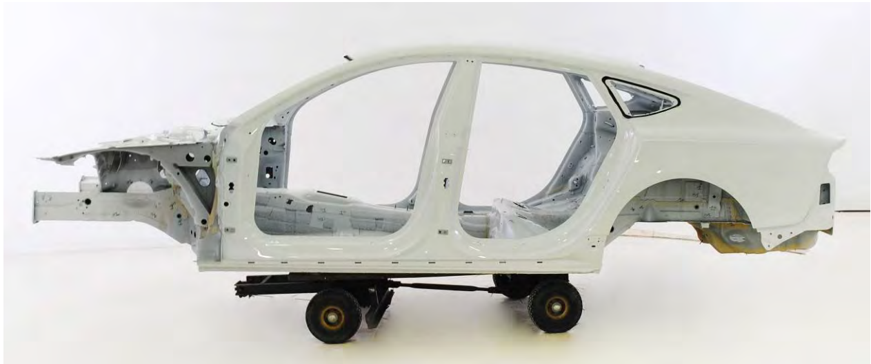
Figure 4.5.8.1.7.d: Audi A7 body-in-white-structure
