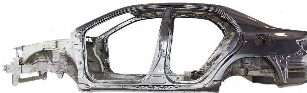
Figure 4.5.8.1.7.b: Toyota Corolla body-in-white structure
