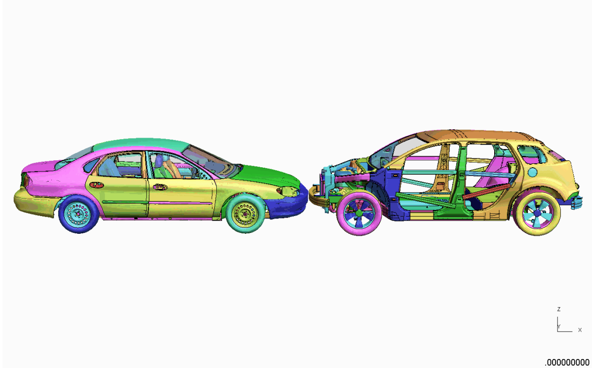
Figure 4.4.9.b: Phase 2 HD vehicle to Ford Taurus crash simulation setup – side view
