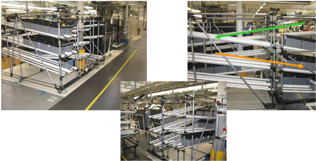
Figure 5.1.b: Shoot technology used to transport small parts
