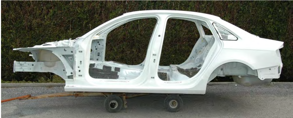
Figure 4.5.8.1.7.c: Audi A4 body-in-white structure
