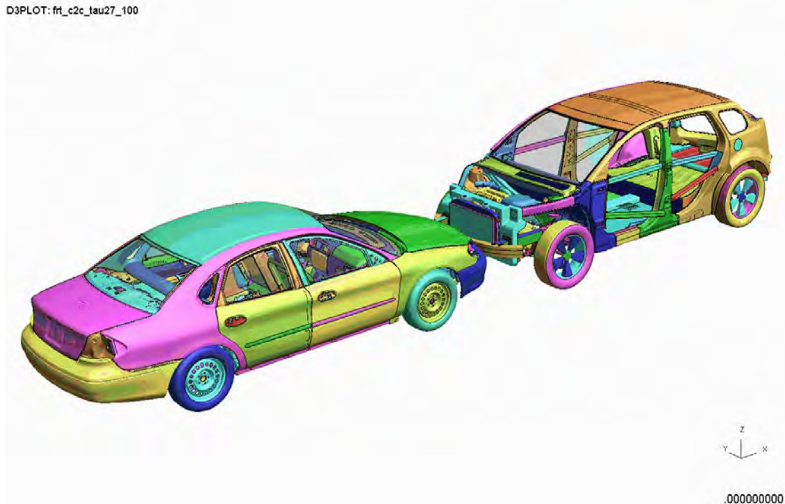
Figure 4.4.9.a: Phase 2 HD vehicle to Ford Taurus crash simulation setup – three-quarter view
