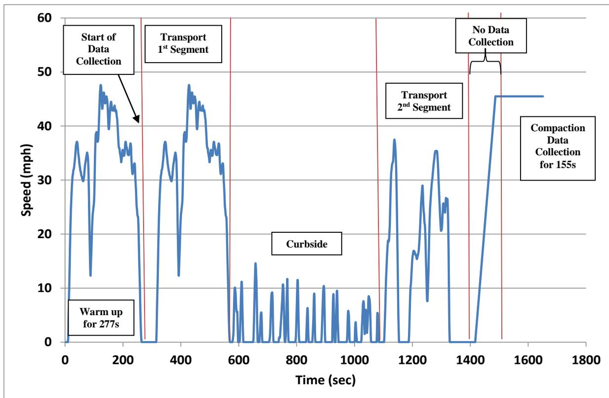
The vehicle was warmed up in the morning over a single iteration of the Refuse Truck Cycle on the fuel that is being tested first on that particular day. Between tests, there was a “hot soak”, where the engine is turned off for about 20 minutes. As discussed above, all tests were conducted as “hot running” tests, with the 277 second warm-up. The road load coefficients and test weight (i.e., 33,520 lbs.) used were the same as that used in the Phase 1 of the refuse hauler testing [28].
