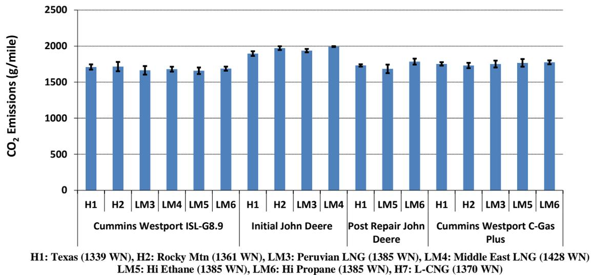
**Figure 3-24 (a-b). Average CO<sub>2</sub> Emissions for the Waste Hauler Transport and Curbside Segments**
