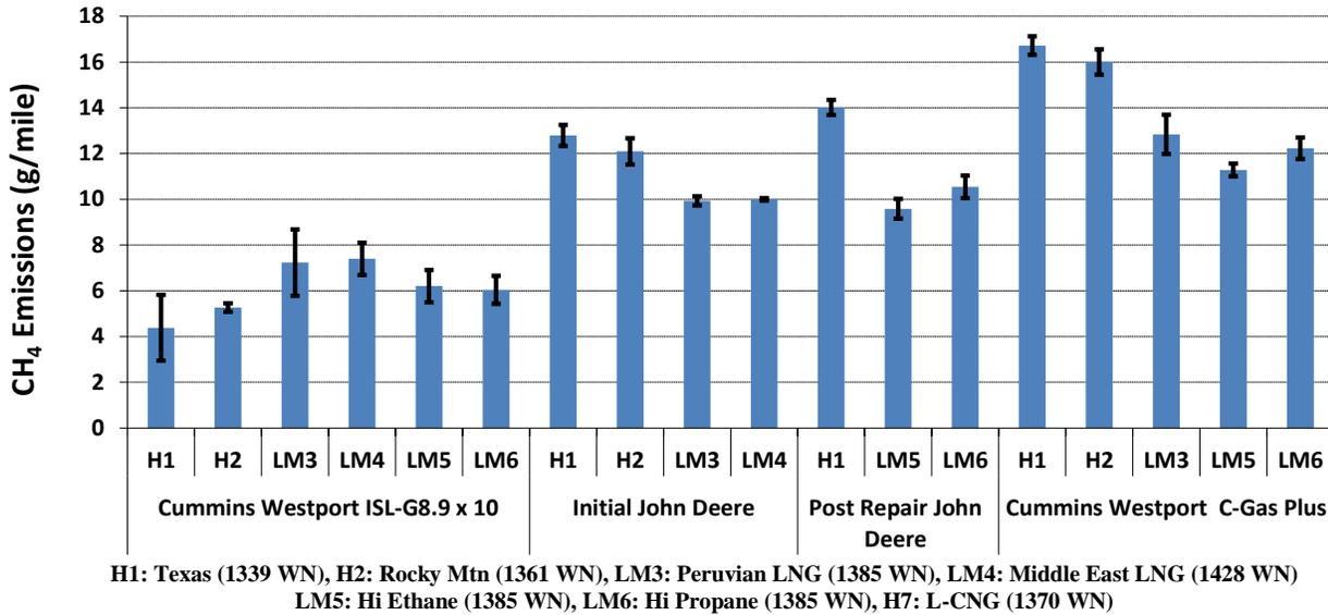
**Figure 3-12 (a-b). Average CH<sub>4</sub> Emissions for Waste hauler Transport and Curbside Segments**
