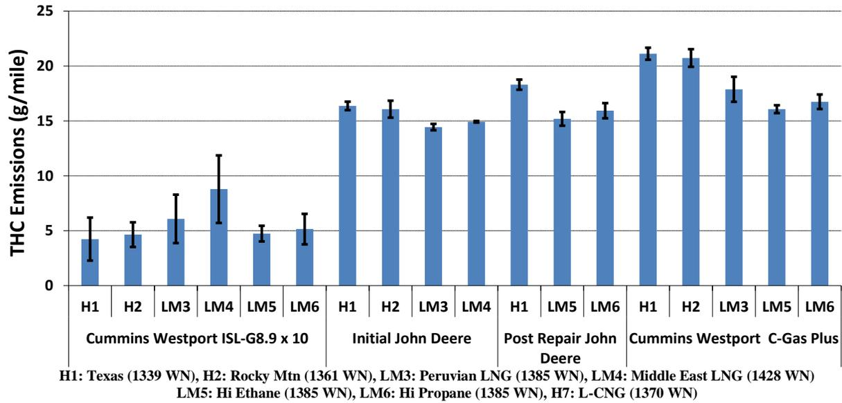
Figure 3-6 (a-b). Average THC Emissions for Waste Hauler Transport and Curbside Segments
