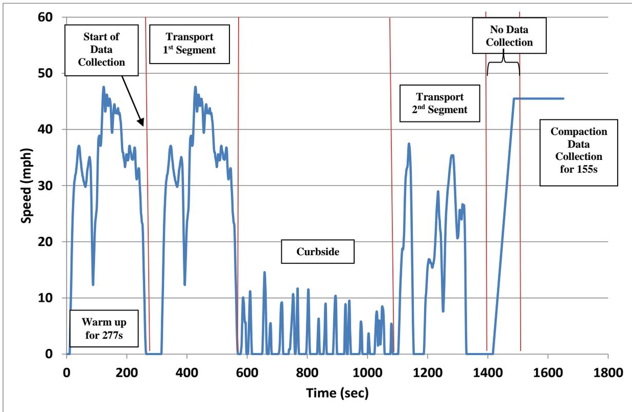
The vehicles were preconditioned at the start of each test day by performing a power map. Between tests, there was a “hot soak”, where the engine is turned off for about 10-15 minutes. As discussed above, all tests were conducted as “hot running” tests, with a single CBD used as the warm-up for the buses and a 277 second warm-up being used by the waste haulers.
