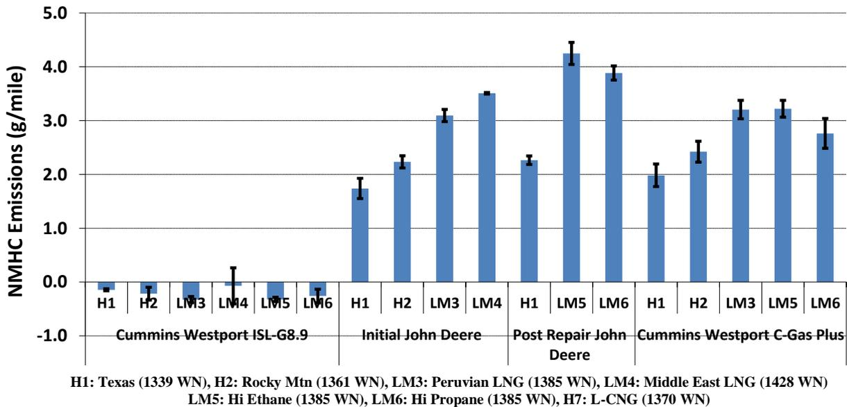
**Figure 3-9 (a-b). Average NMHC Emissions for Waste hauler Transport and Curbside Segments**
