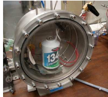
Photo 4.16 Accumulation volume where refrigerant annual leak is measured
