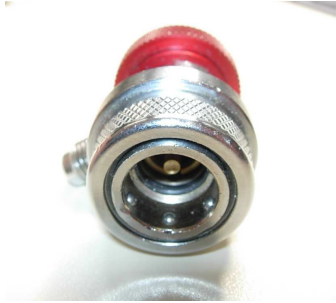
Photo 4.3 Quick coupler - Connection with moving rod by screwing fastened with clips.
