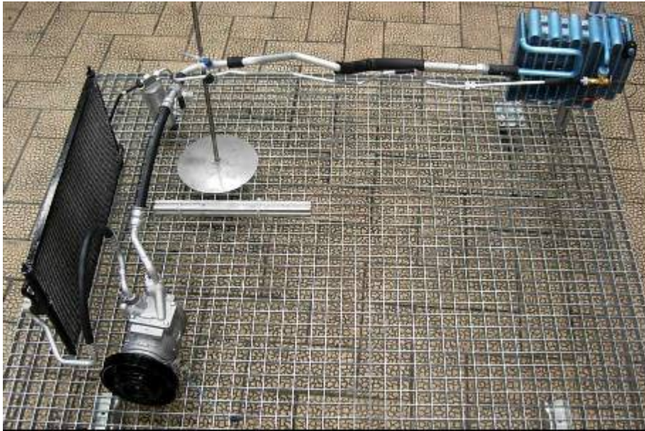
Photo 1.5 Assembled MAC system D.
