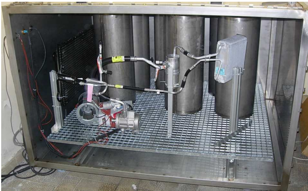
Photo 1.1: Installation of MAC system in mini-shed.
