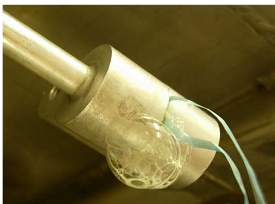
Photo 4.21 Leak detection with Soap Bubble (1200 g/yr).
