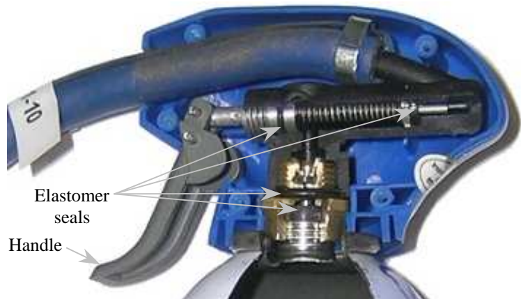
Photo 4.15 Sectional view of a push button valve.
