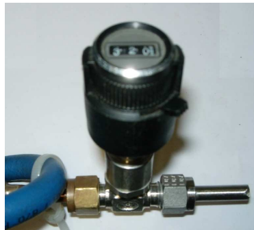
Photo 4.2 Leak valve with micro counter.
