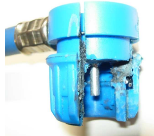
Photo 4.6 Quick coupler - connections with fixed rod fastened with clips.
