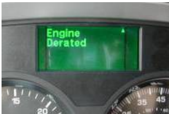
Figure 10 - Driver Information Center Engine De-rated Message
