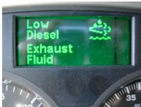
Figure 9 - Driver Information Center Low DEF Message
