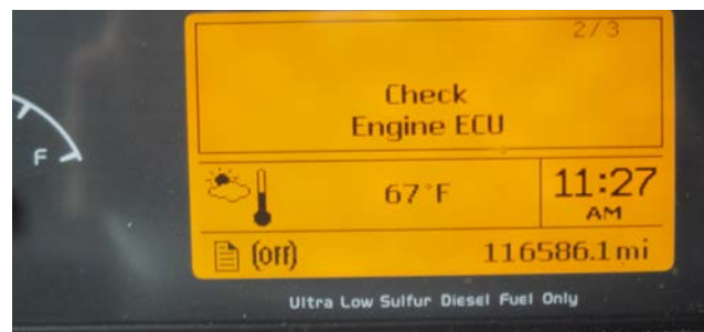
Figure Volvo-10: Volvo’s Driver Information Display Indicating to Check ECU
