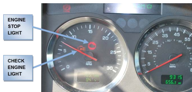
Figure Cummins 14.9-4: Stop Engine Lamp and Check Engine Light
