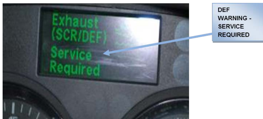
Figure Cummins 14.9-8: DIC Message – Exhaust (SCR/DEF) Service Required
