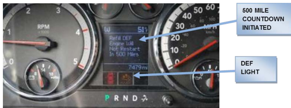
Figure Cummins 6.7- 4: Example of Message Alert, 500 Mile Countdown
