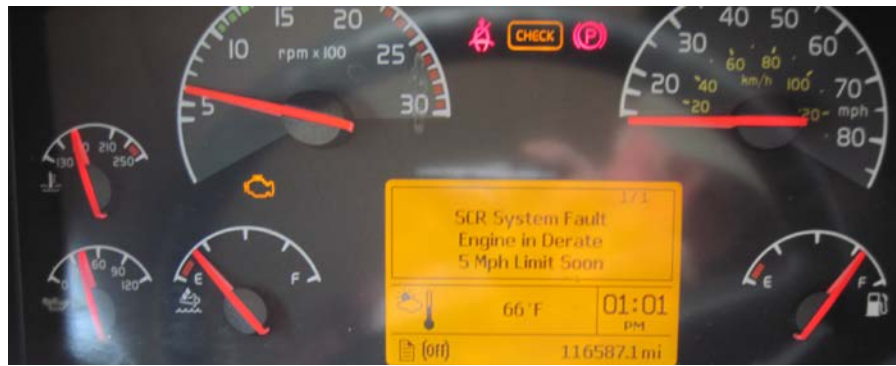
Figure Volvo-11: Volvo Driver Information Display Indicating 5 Mph Derate
