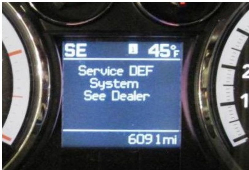
Figure Cummins 6.7-6: Tampering Message
