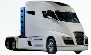
Tractor* Range: 500-1,000 miles Battery: 250 kWh+100 kg H2
