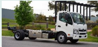
Cabover Chassis Range: 100 miles Battery: 136 kWh
