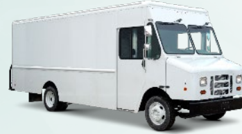
Step Van Range: 90-120 miles Battery: 96-128 kWh
