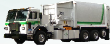
Refuse Truck Range: 80 miles Battery: 352 kWh
