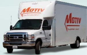
Conventional Chassis Range: 100-230 miles Battery: 106-325 kWh
