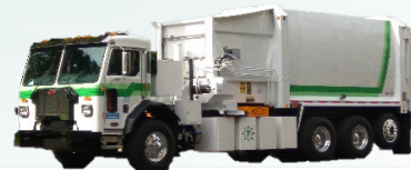
Refuse Truck Range: 80 miles Battery: 352 kWh
