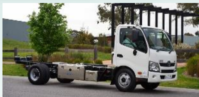
Cabover Chassis Range: 100 miles Battery: 136 kWh
