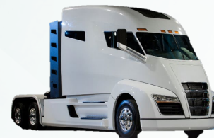
Tractor* Range: 500-1,000 miles Battery: 250 kWh+100 kg H2
