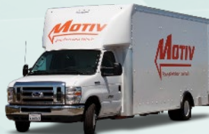
Conventional Chassis Range: 100-230 miles Battery: 106-325 kWh
