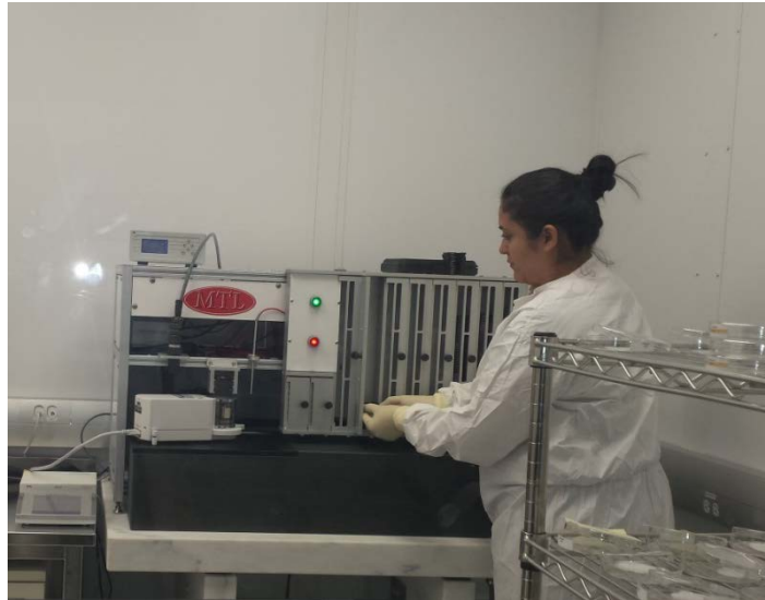
Figure II-2. An operator loads filters on ARB's automated filter weighing system.
