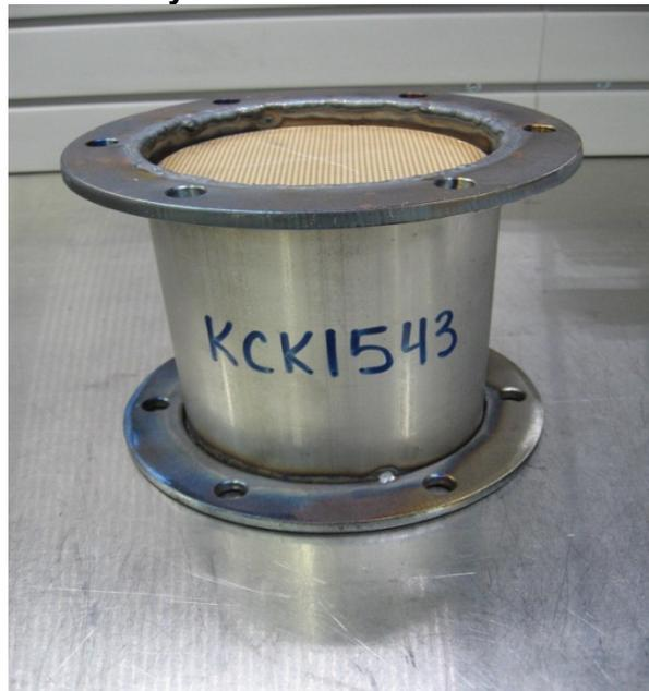
Without the GPF, both vehicles had fairly high FTP PM emissions and would need further improvements to meet the 3 mg/mi standard. The emission reductions from GPF testing are shown in Table 3. On the FTP, an 88% reduction was observed for both vehicles and brought
