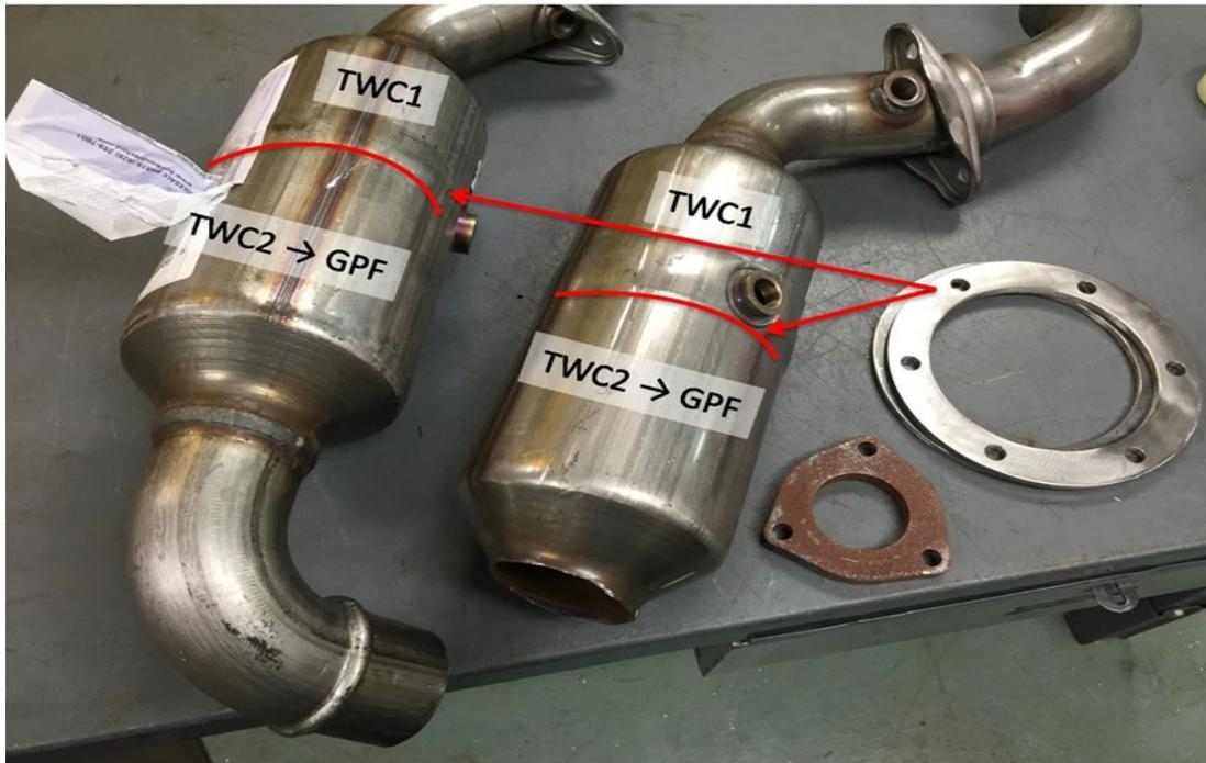
**Figure 4 - Malibu Underfloor Catalyzed GPF**
