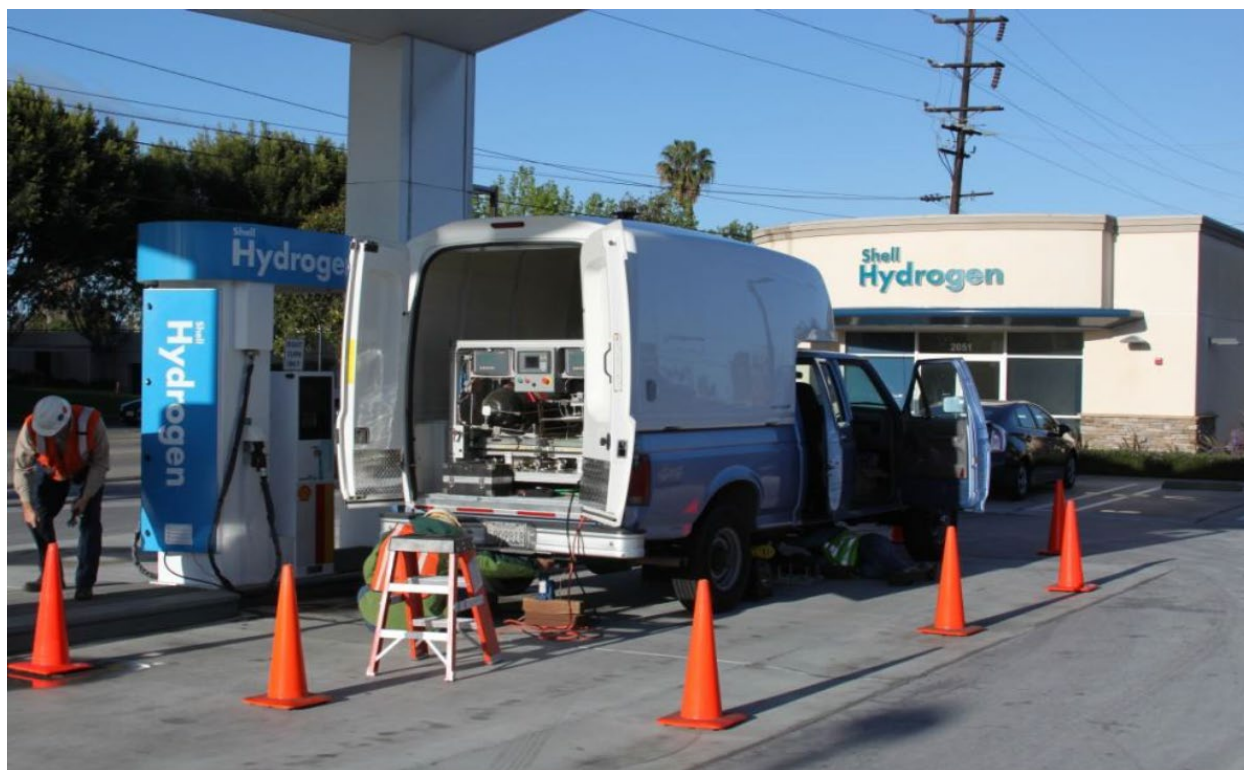
Figure 36 - HFS Device Being Set-Up to Perform a Station Accuracy Confirmation Test
