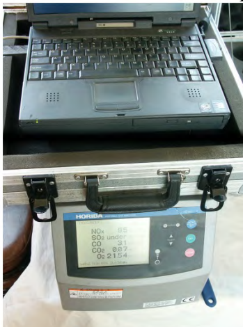
Figure E-3 Setup Showing Gas Analyzer with Computer for Continuous Data Logging
