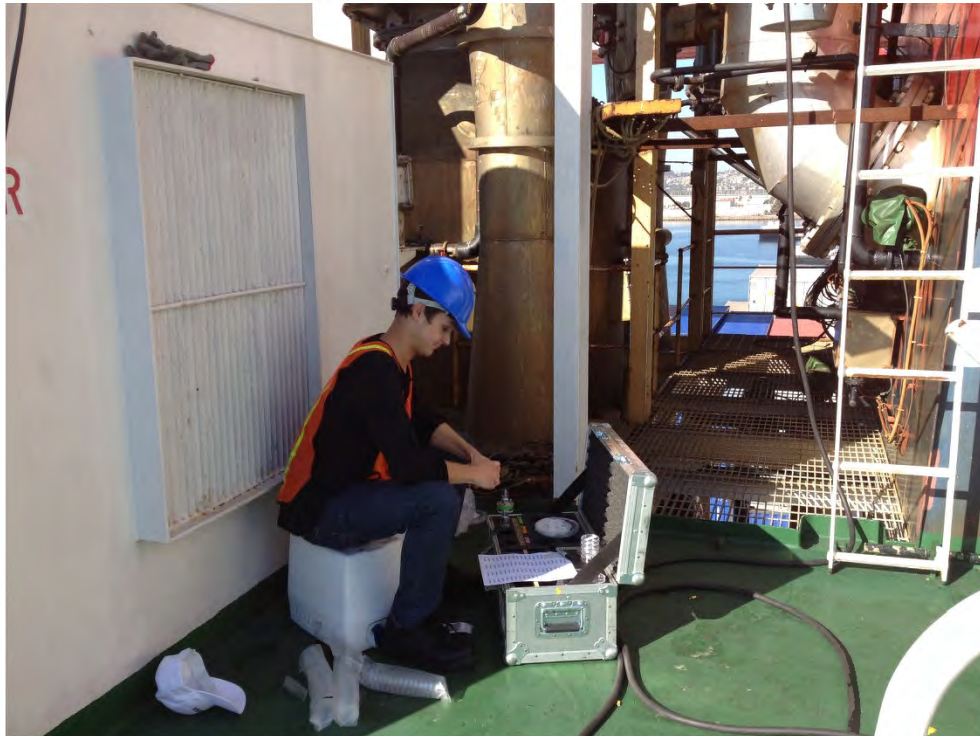
Figure 3-4 PM sampling and filter change out during testing.
