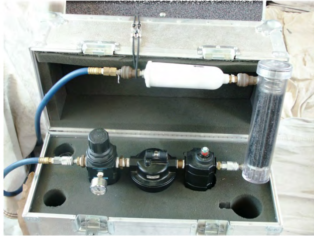
Figure E-2 Field Processing Unit for Purifying Dilution Air in Carrying Case
