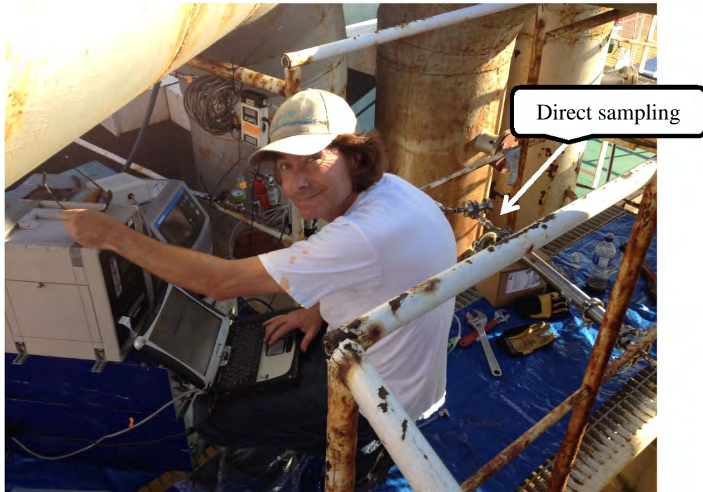
Figure 3-3 Dilution system and measurement layout on the auxiliary engine exhaust stack
