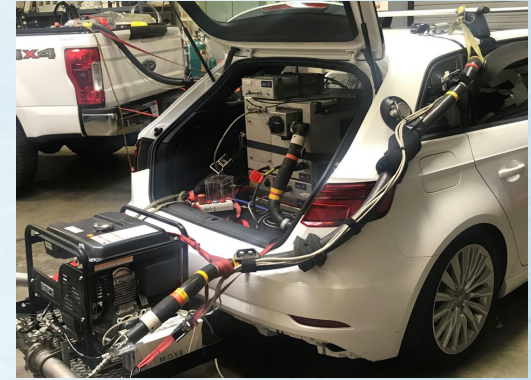
PEMS Testing Setup
