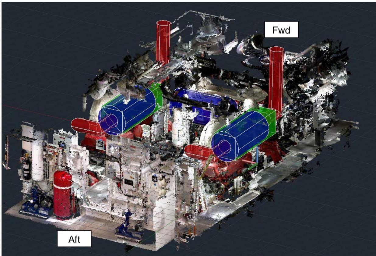
*Figure 24. Special Use Vessel Retrofit Arrangement*
