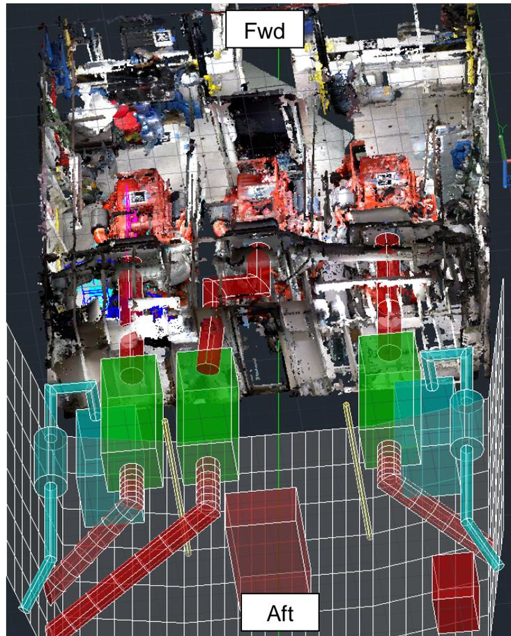
*Figure 21. Crew Supply Boat Retrofit Arrangement*
