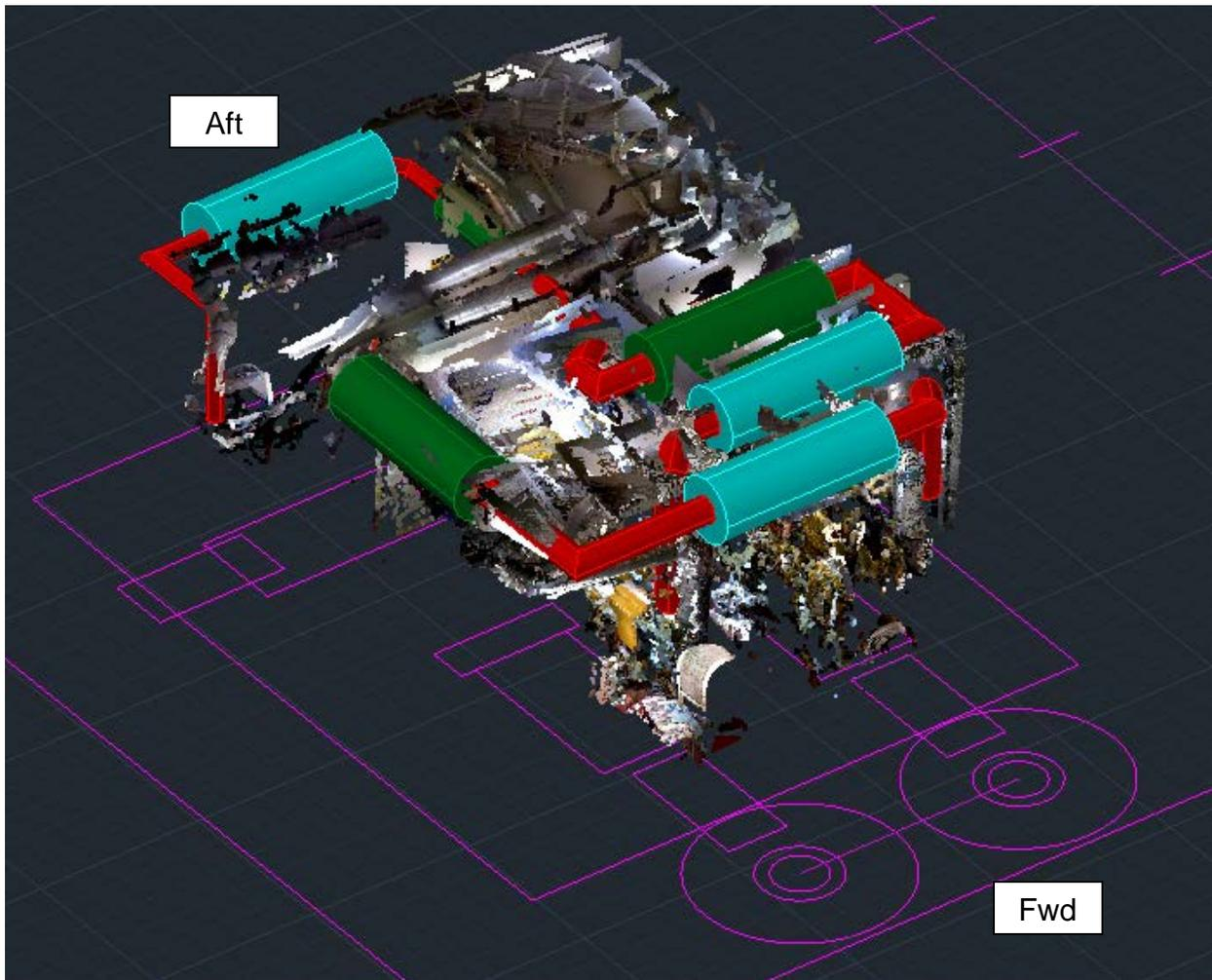
*Figure 3. Barge Stbd Engine Room Retrofit Arrangement*
