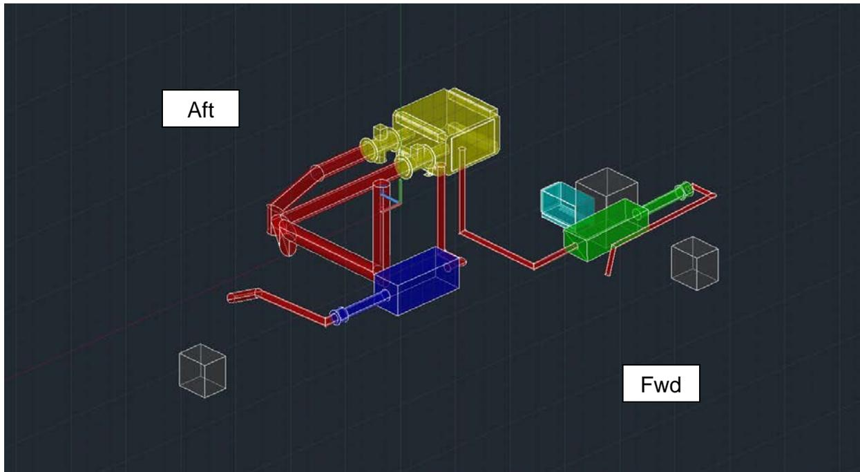
*Figure 8. Dredge Thruster and Generator Engine Retrofit Arrangement with Point Cloud Suppressed*
