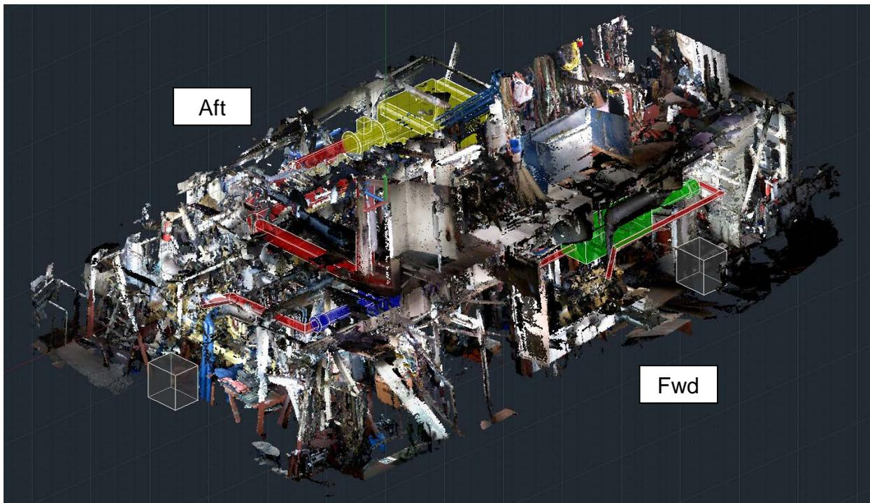
*Figure 7. Dredge Thruster and Generator Engine Retrofit Arrangement*
