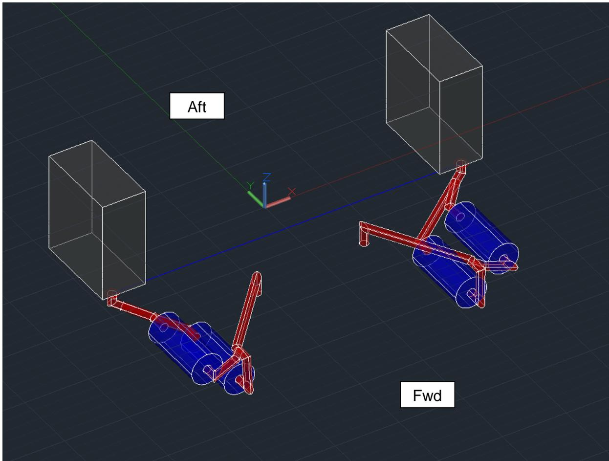
*Figure 13. Slow Speed Ferry Retrofit Arrangement with Point Cloud Suppressed*
