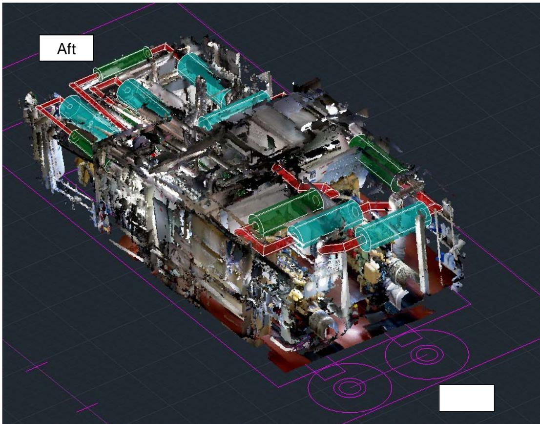
Figure 1. Barge Port Engine Room Retrofit Arrangement
