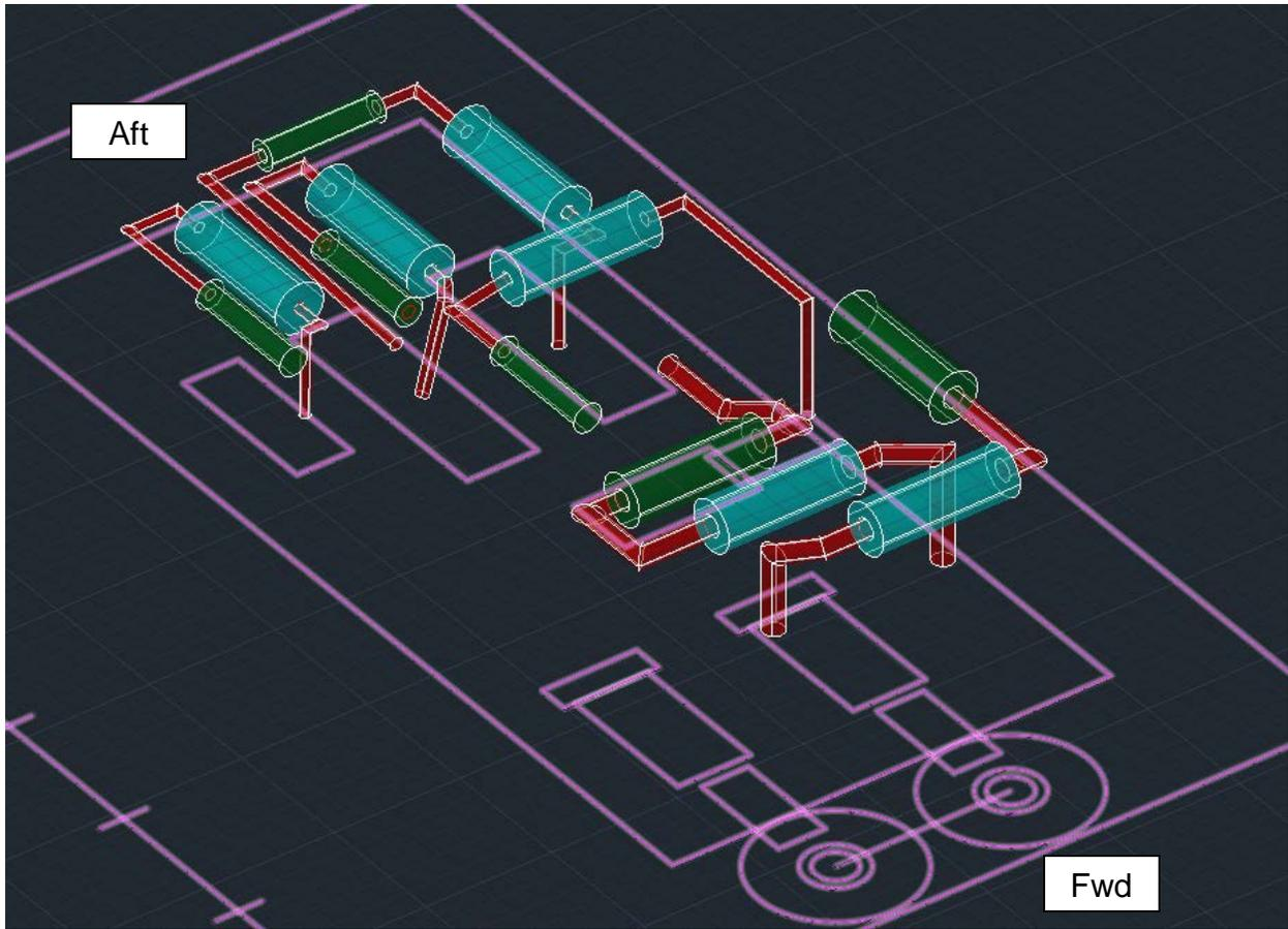
*Figure 2. Barge Port Engine Room Retrofit Arrangement with Point Cloud Suppressed*
