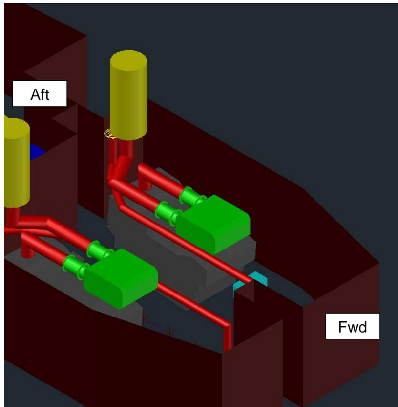
*Figure 18. Ship Assist Tug Repower Arrangement*
