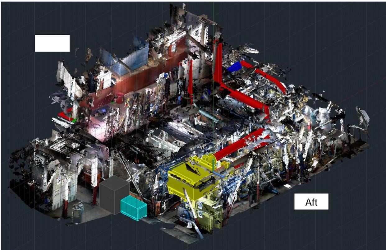
*Figure 5. Dredge Pump/Winch Engine Repower Arrangement*
