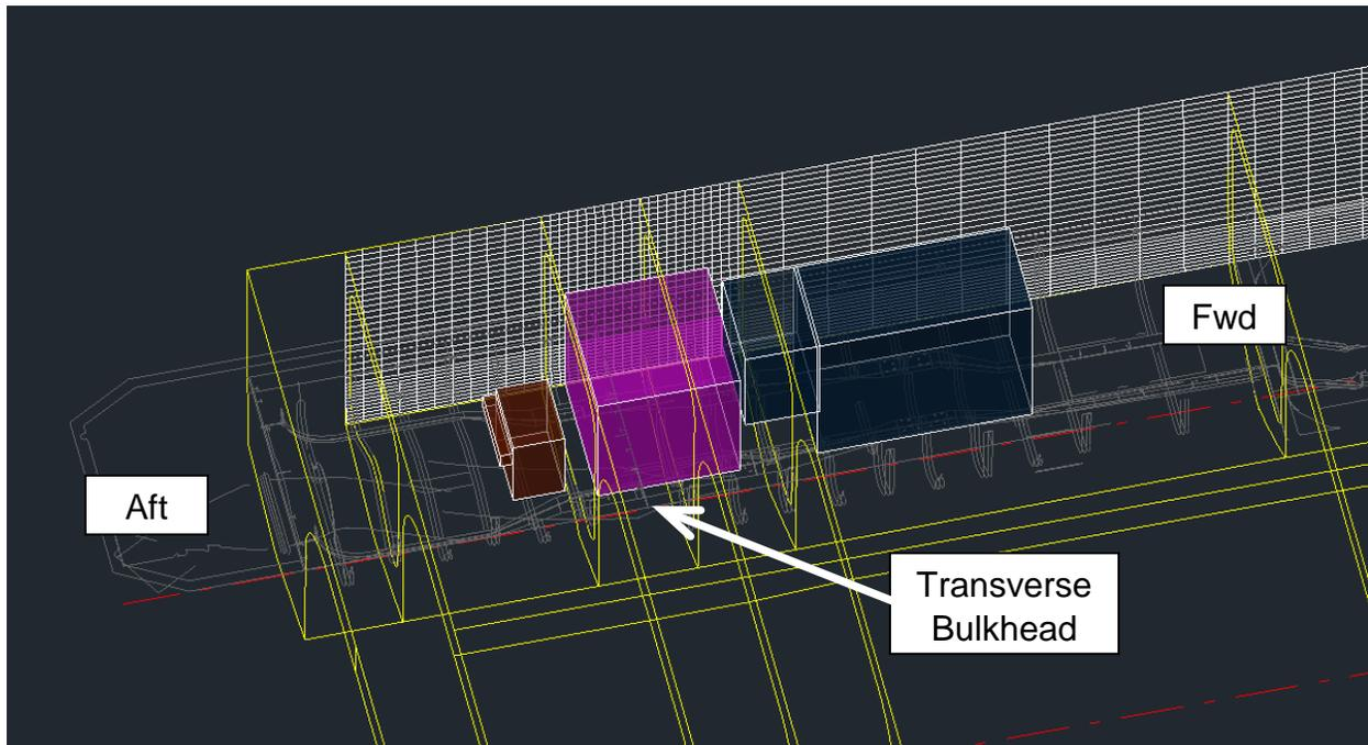
*Figure 16. High Speed Ferry Repower Arrangement (Port Hull Shown)*
