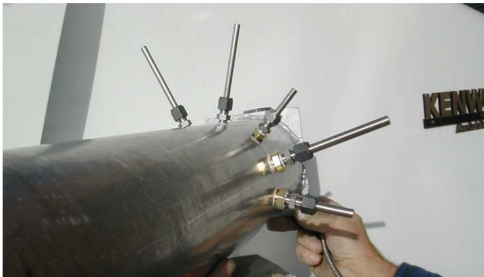
Figure II-6– Individual probes to emissions equipment
