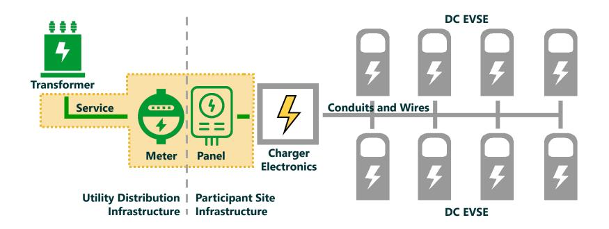
Program covers costs associated with service drop, meter, panel, and circuit dedicated to EV charging. Make-ready ends at interconnection point with customer charging equipment providing AC service.
