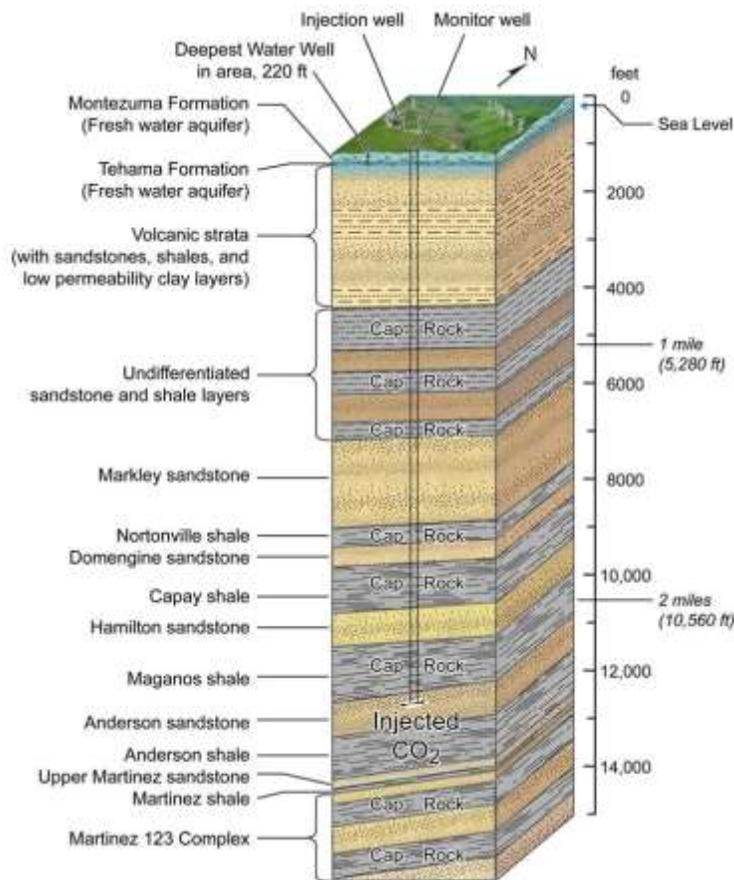
**Figure A2.** General Stratigraphy at the Montezuma Hills site. The Domengine, Capay and Maganos are present, but are significantly deeper than to the east at the King Island and Thornton sites.
