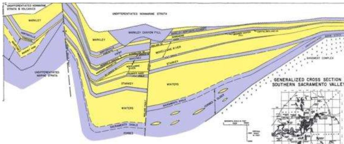
**Figure 2.1.** Cross-section interpretation of the stratigraphy in the southern Sacramento Basin, showing geologic units consisting of predominantly sandstone (in yellow) and shale (in gray). (Downey and Clinkenbeard, 2005).
