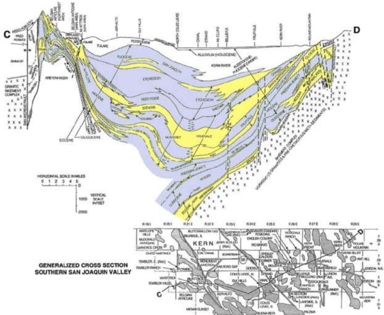
**Figure 2.8.** Cross-section interpretation of southern San Joaquin Basin stratigraphy, showing geologic units that consist predominantly of sandstone (in yellow) and shale (in gray) (Downey and Clinkenbeard, 2005).
