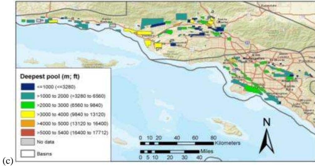
**Figure 1.17.** Deepest average hydrocarbon pool depth in each field in each major oil and gas basin in California listed in DOG (1982a and 1992) and DOGGR (1998): (a) Sacramento Basin, (b) Santa Maria Basin to the southwest and central and southern portion of the San Joaquin Basin to the northeast, and (c) Santa Barbara-Ventura Basin to the north and Los Angeles Basin to the southeast.
