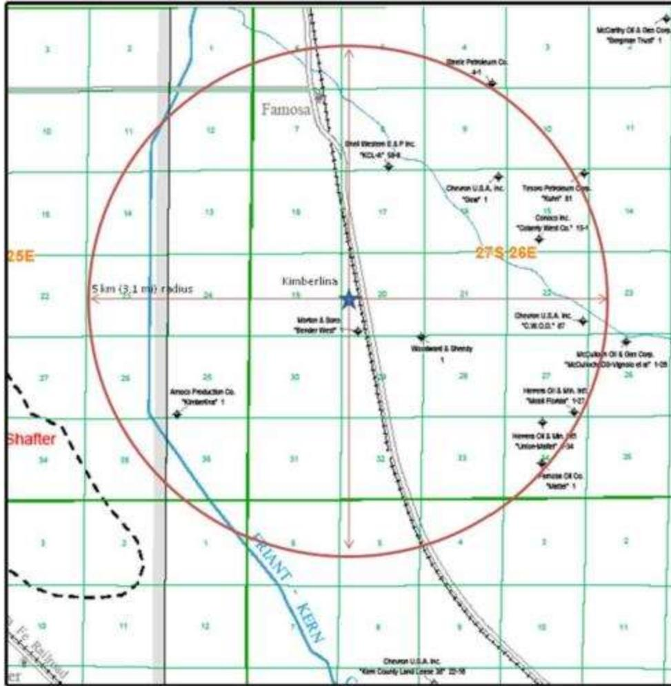
**Figure 2.16.** Locations of known exploration borings and active wells within a 5 km radius of the Kimberlina site.
