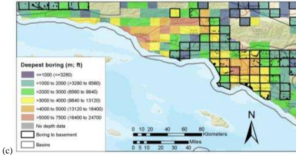
**Figure 1.18.** Deepest prospect boring and whether a prospect boring encountered basement in each township prior to 2010 (data from DOG 1982b and 1982-1992, and DOGGR 1993-2010): (a) Sacramento Basin, (b) Santa Maria Basin to the southwest and central and southern portion of the San Joaquin Basin to the northeast, and (c) Santa Barbara-Ventura Basin to the north and Los Angeles Basin to the southeast.
