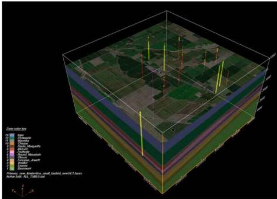
**Figure 2.14.** Sub-model centered on the Kimberlina site, extending 10 x 10 km (6 x 6 mi). The yellow vertical lines are cemented boring segments and the red vertical lines are uncemented segments. (Wagoner, 2009).
