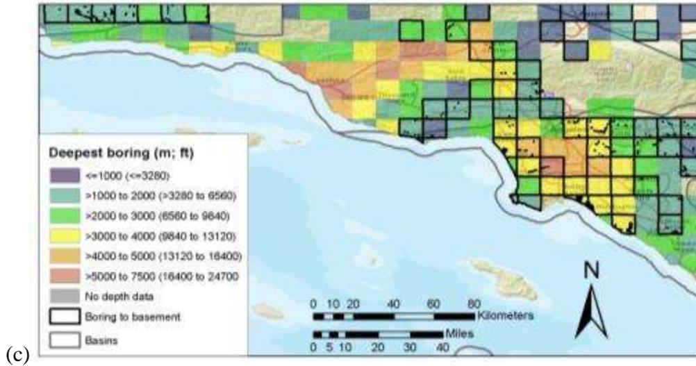
**Figure 1.16.** *Deepest prospect well and whether a prospect well encountered basement in each township prior to 1981 (data from DOG 1982b): (a) Sacramento Basin, (b) Santa Maria Basin to the southwest and central and southern portion of the San Joaquin Basin to the northeast, and (c) Santa Barbara-Ventura Basin to the north and Los Angeles Basin to the southeast.*
