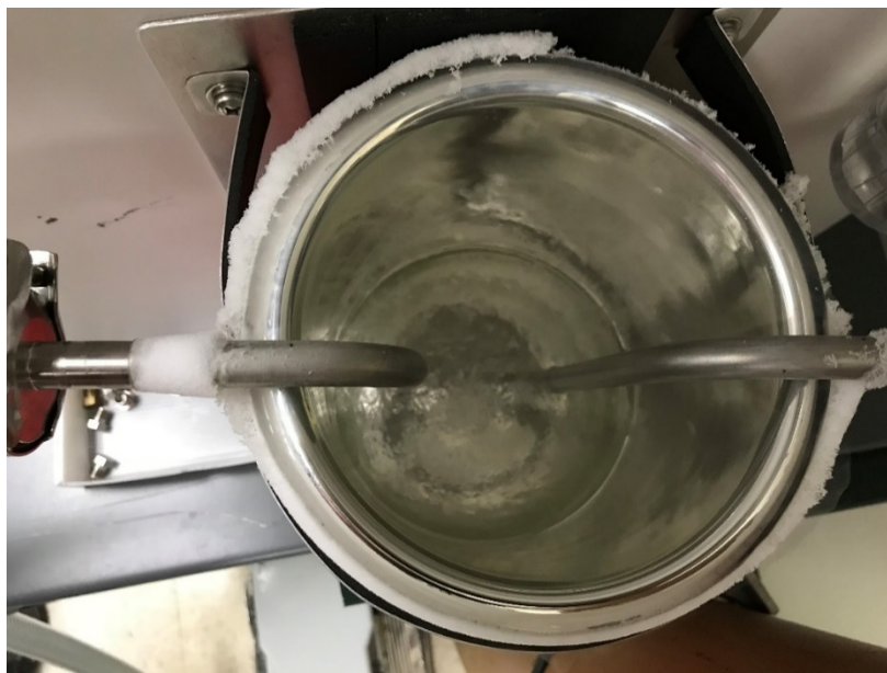
Figure 5. U-trap Inside Liquid Nitrogen Dewar
