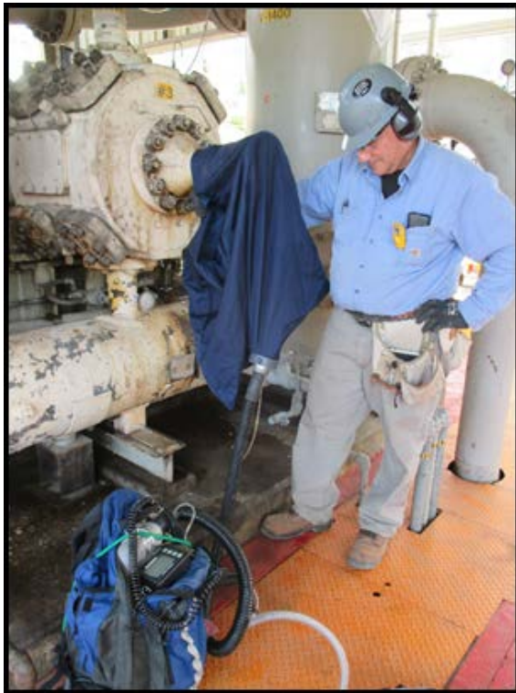
Figure 2-4 Emission Testing with the Hi Flow Sampler
