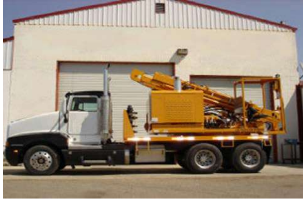
Guardrail Installer (Drop Hammer)
