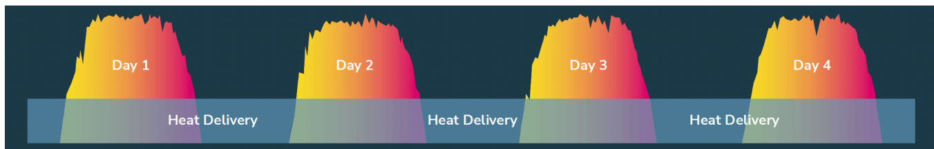
Intermittent charging from wind and sun, continuous industrial heat delivery
