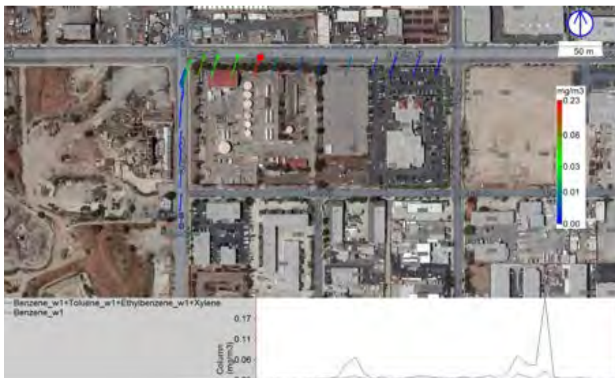
Figure 32. Emission on October 3, 10:10-10:12, from the treatment site denoted “TreatmentSite_OrangeAve_ESpringSt_SE” in the result section. Each measured spectrum is represented with a point, with color and size indicating the evaluated integrated vertical BTEX column according to the logarithmic color bar. The BTEX (black) and benzene (blue) column by distance driven through the plume is also shown in the lower part of the figure. A line from each point indicates the direction from which the wind is blowing. The wind was blowing from south at 3.5 m/s.
