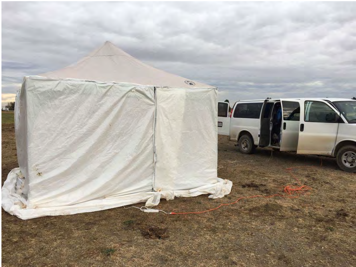
Gas well No. 095-20708 under "tent chamber" for testing. Photographer: Eric Lebel
