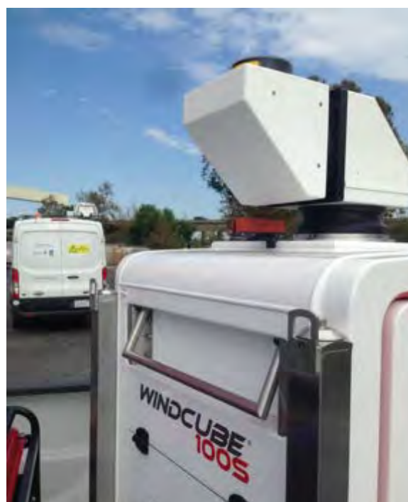
Figure 7. The WindCube 100S (Leosphere) LIDAR used for wind profile measurements in this project.
