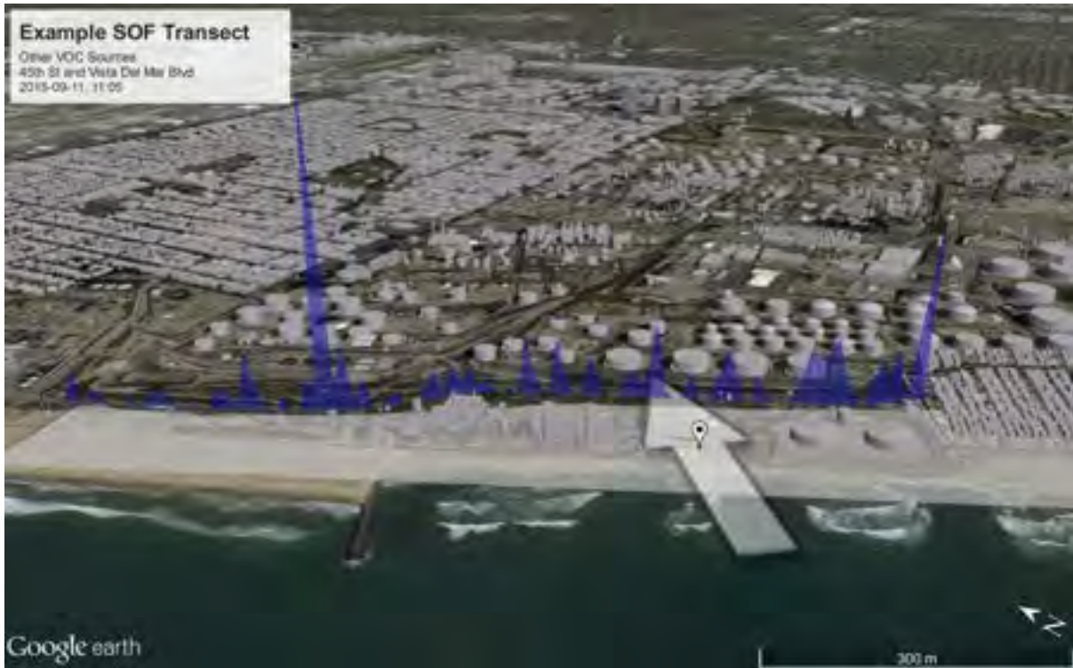
Figure 23. Example of a SOF measurements of a VOC source west of Vista Del Mar Blvd in Long Beach, 11 September 2015, 11:05. Alkane column is shown as a blue curve with apparent height proportional to gas column (10 m equivalent to 1 mg/m 2 , max 30 mg/m 2 ). Wind direction during the measurement is indicated by the white arrow, measured with the FluxSense 10m wind mast. Map from Google Earth™ 2016.
