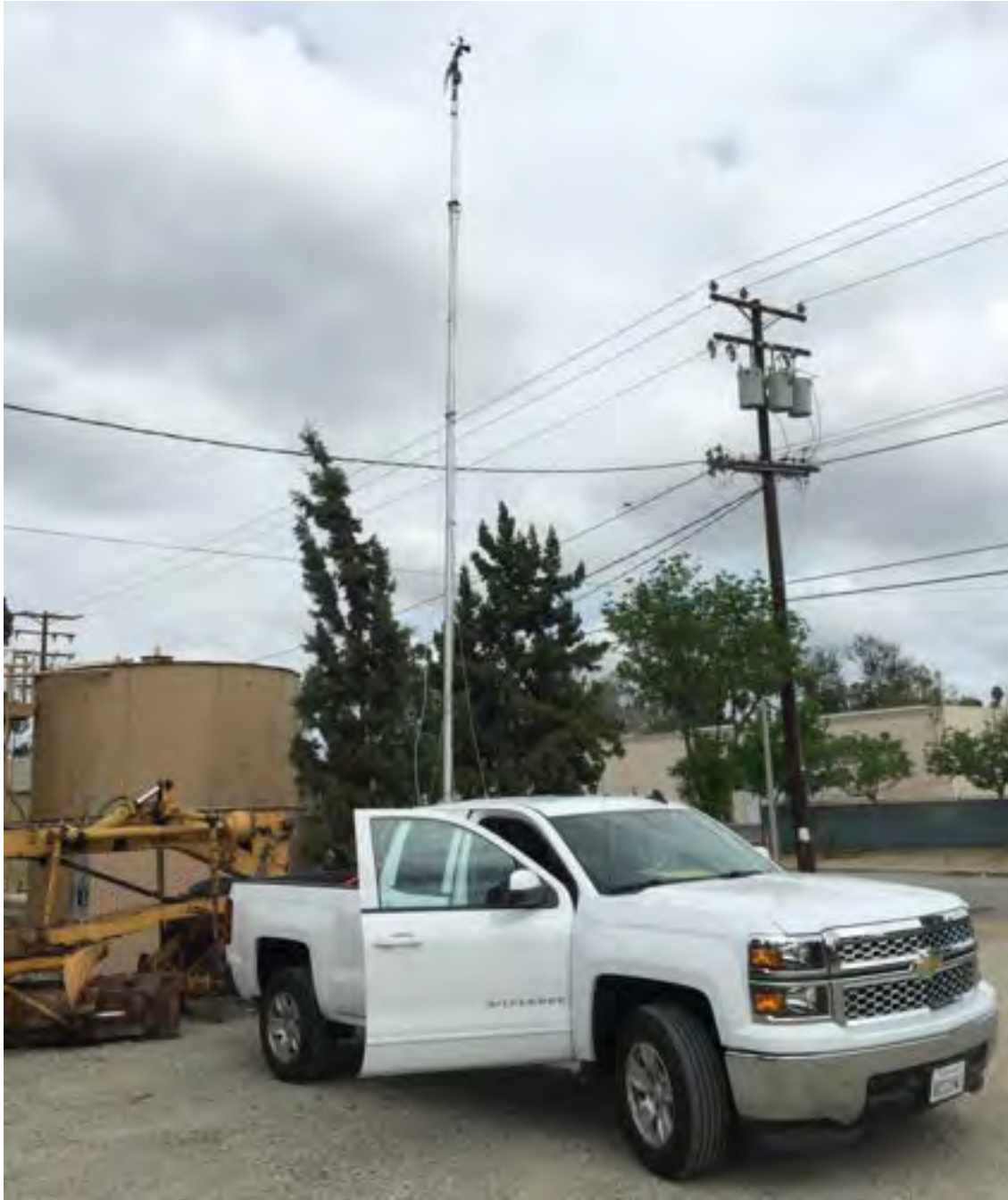
Figure 11. FluxSense mobile wind mast mounted on the bed of pick-up truck. An RM Young anemometer is used throughout the project. The mast could be erected from 3 to 10 m.
