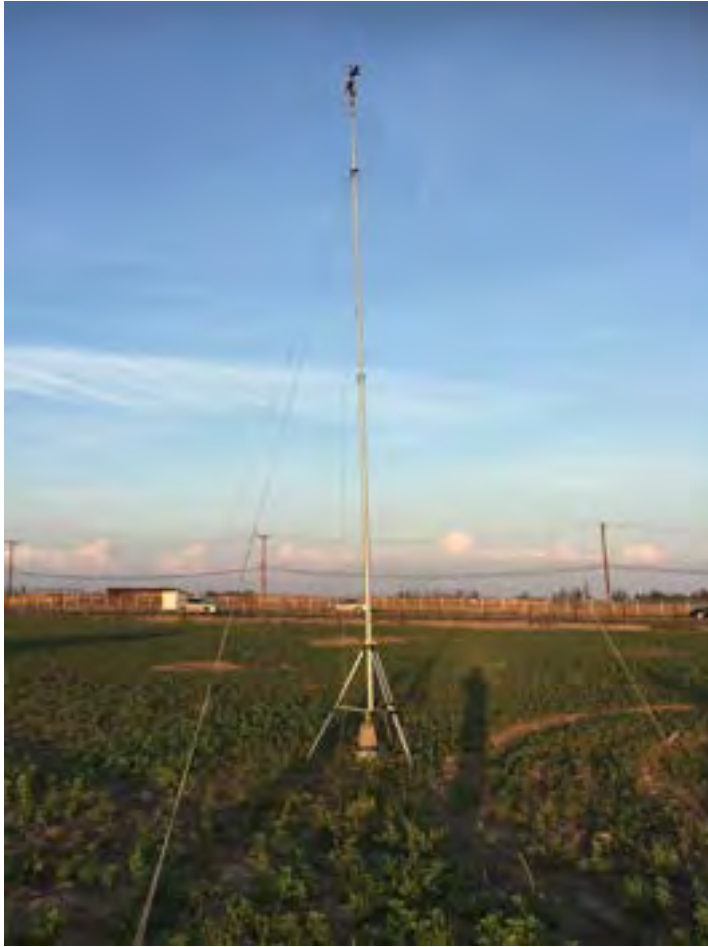
Figure 8. The FluxSense mobile wind mast used in the 2015 SCAQMD survey with an RM Young anemometer mounted on top. The mast could be erected from 3 to 10 m.
