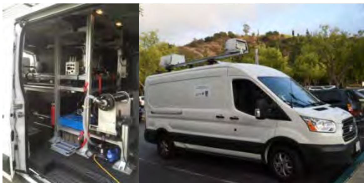
Figure 3. Internal and external view of the FluxSense mobile lab.
