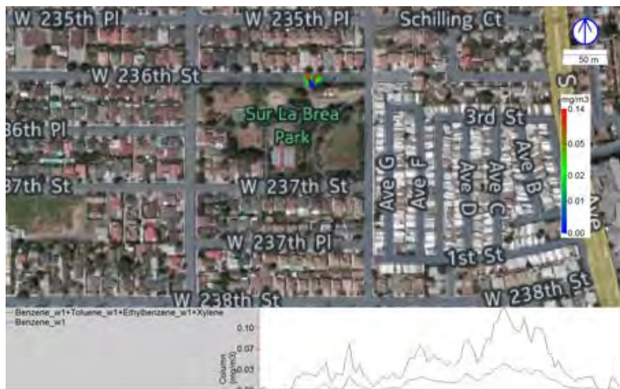
Figure 27. Emission from derricks with associated tanks (main source) at Sur La Brea Park, denoted “Wells_WalnutSt_W236thSt_SW” in the result section, on October 25, 1:35 -1:41 pm. BTEX levels up to 140 \mu\text{g}/\text{m}^3 was observed on the nearby street, of which 45 \mu\text{g}/\text{m}^3 was benzene. Wind speeds were low at the time, about 1-2 m/s. Each measured spectrum is represented with a point, with color and size indicating the evaluated integrated vertical BTEX column according to the logarithmic color bar. The BTEX (black) and benzene (blue) column by distance driven through the plume is also shown in the lower part of the figure. A line from each point indicates the direction from which the wind is blowing.
