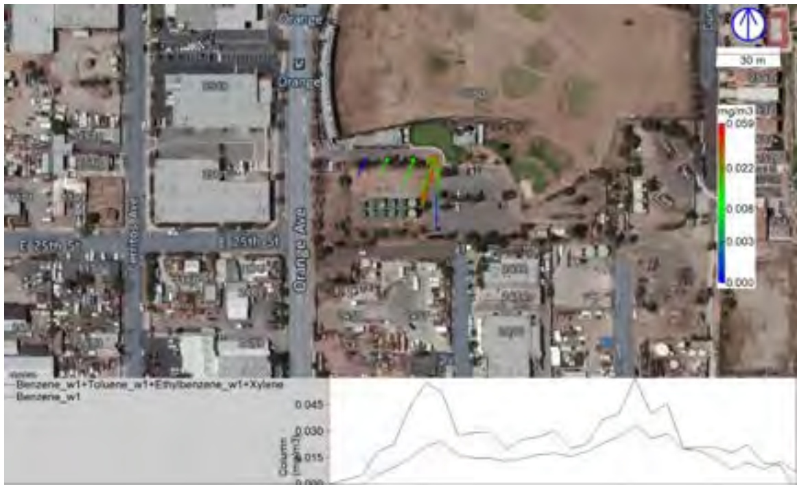
Figure 34. Emission on October 15, 1:46-1:48 pm, from the tank farm denoted “TankFarm_OrangeAve_E25thSt_NE” in the result section. Each measured spectrum is a point, with color and size indicating the evaluated integrated vertical BTEX column according to the logarithmic color bar. The BTEX (black) and benzene (blue) column by distance driven through the plume is also shown in the lower part of the figure. A line from each point indicates the direction from which the wind is blowing. Wind speed was about 5 m/s, coming from SSW.
