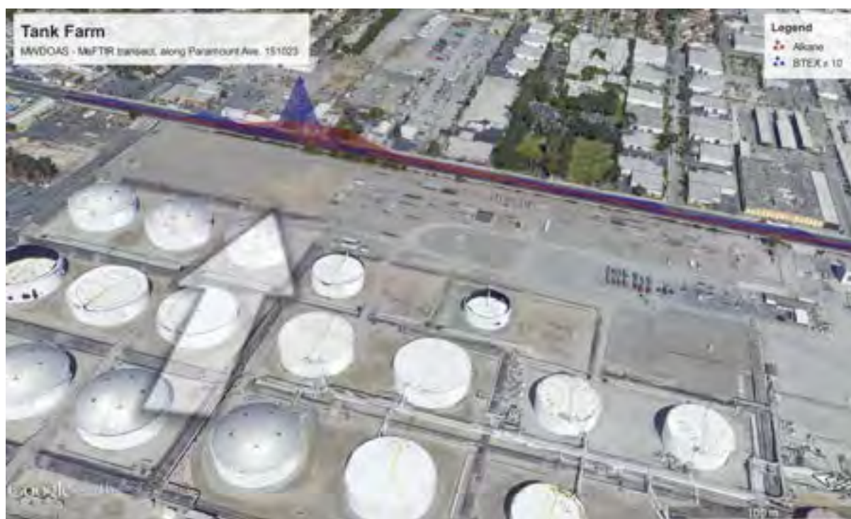
Figure 18. Example of a MWDOAS/MeFTIR measurement of a Tank Farm along Paramount Ave, Paramount 23 October 2015, 12:17. Alkane concentration is shown as a red curve and the BTEX is shown as a blue curve. The BTEX have been magnified x 10 for visibility. Wind direction during the measurement, indicated by the white arrow, was measured with the FluxSense 10m wind mast. Map from Google Earth™ 2016.
