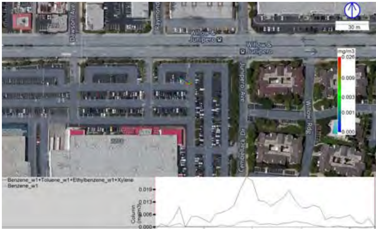
Figure 35. Emission on Oct 15, 5:02-5:04 pm, from the gas station at Cherry Ave. and E Willow St. in Signal Hill. Each measured spectrum is represented with a point, with color and size indicating the evaluated integrated vertical BTEX column according to the logarithmic color bar. The BTEX (black) and benzene (blue) column by time standing still in the plume is also shown in the lower part of the figure. A line from each point indicates the direction from which the wind is blowing. Wind speed was about 2.5 m/s, coming from W, and the distance from sample position to the source was 160 m.
