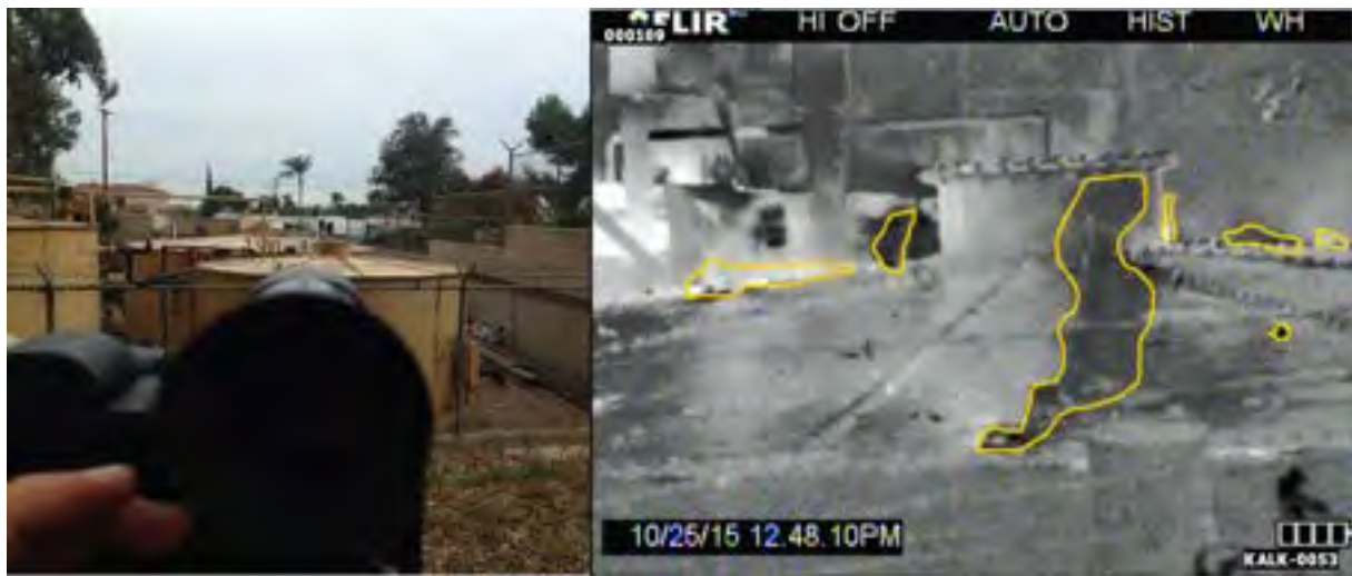
Figure 28. After MWDOAS detected the BTEX plume at the site by Sur La Brea Park (Figure 27), an infrared gas camera (FLIR) was used to visualize the observed emissions. To the left is a photo of the site, with the gas camera in the foreground. To the right a snapshot from the infrared camera is shown, with emerging gas enhanced by a yellow line here. VOC was being emitted from many leaks on the tank roof and pipes, and the gas is seen as black or white against the grey background.
