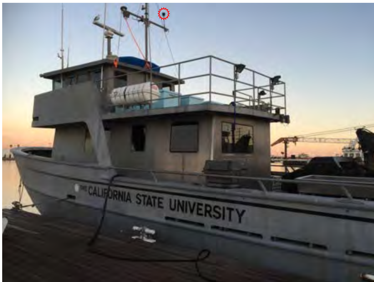
Figure 12. The research vessel for sea-based SOF measurements during the SCAQMD 2015 survey. The sonic wind sensor encircled in red at the top.
