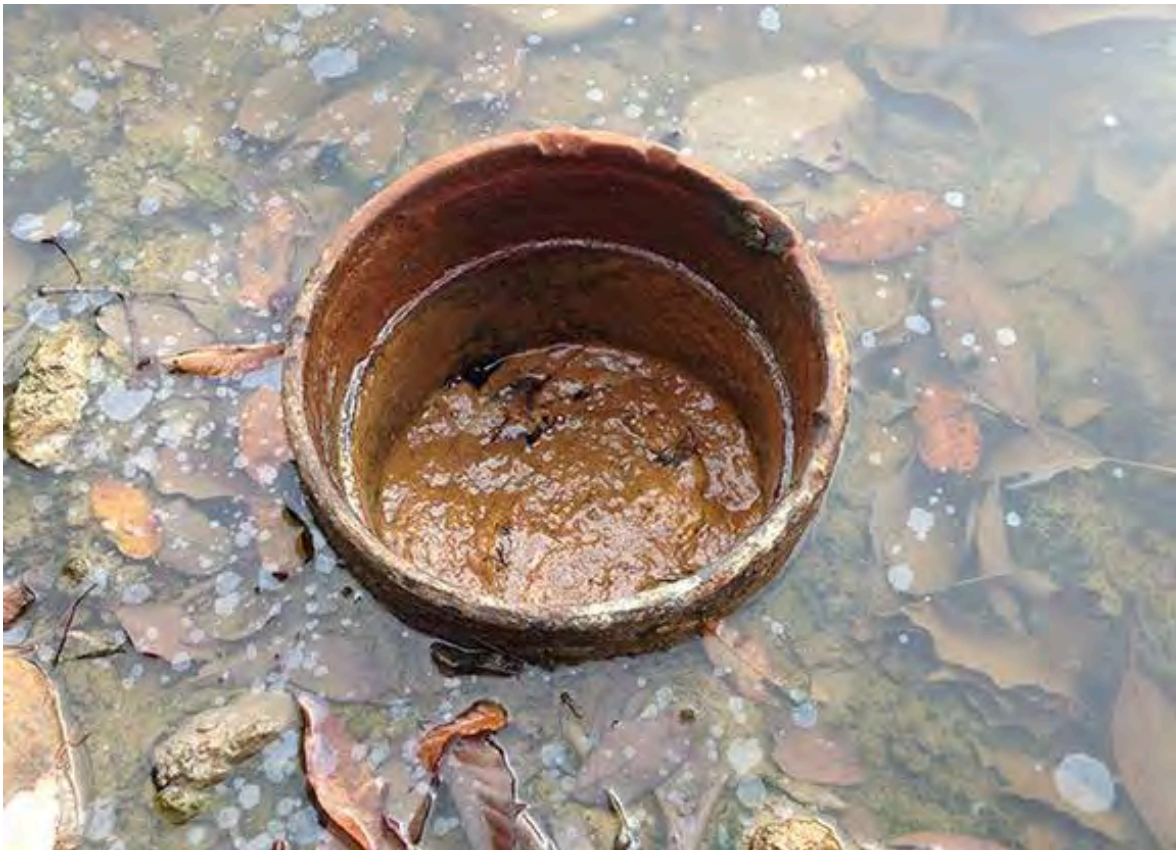
A well pipe emerges from the ground in the Allegheny National Forest in northwestern Pennsylvania. Researchers covered pipes from 19 wells with instruments to measuring gases emitted by the well. (Photo courtesy of Mary Kang, Department of Civil and Environmental Engineering)
