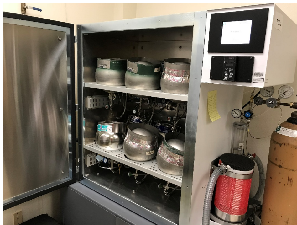
Figure 1. TO-Clean Canister Cleaning System
