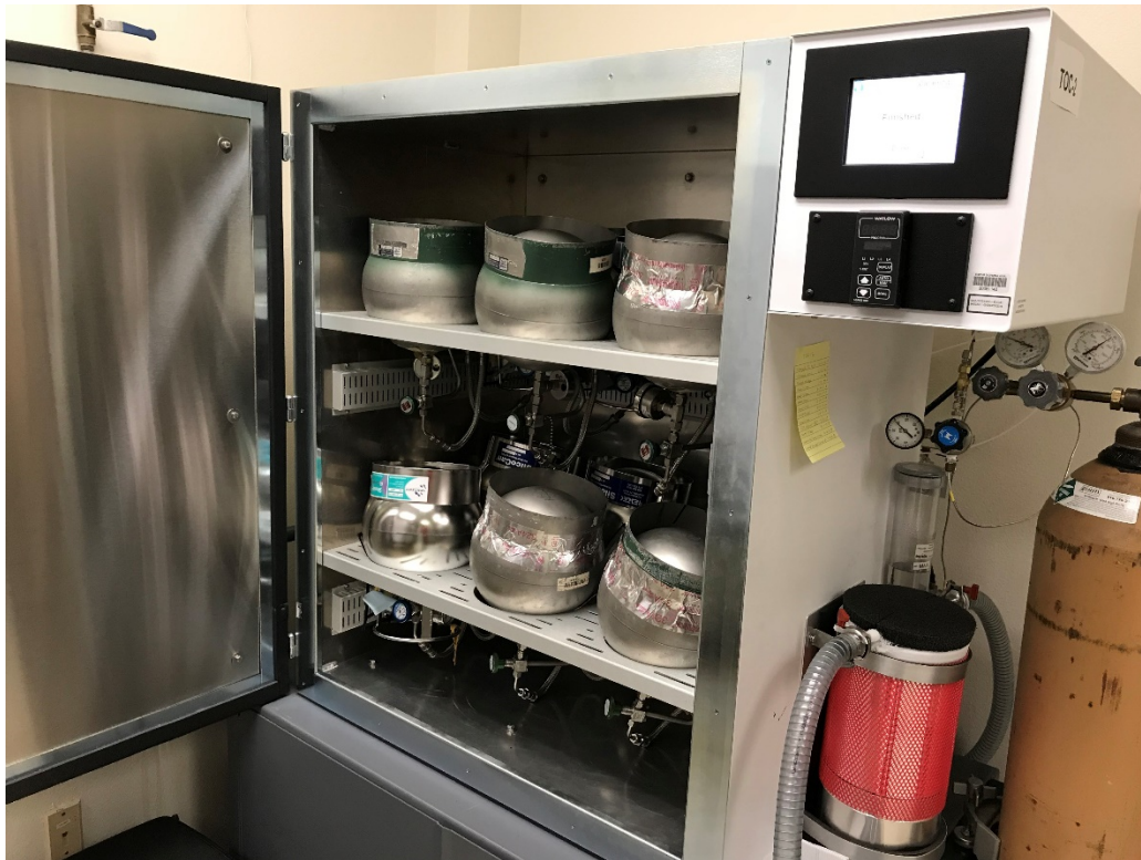
Figure 1. TO-Clean Canister Cleaning System
