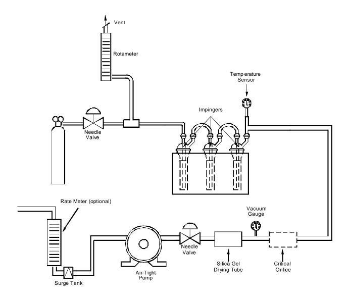
Figure 16A-4. Recovery Check Gas Sampling Train.
