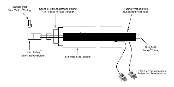
Figure 16A-2. Angled Sampling Probe.
