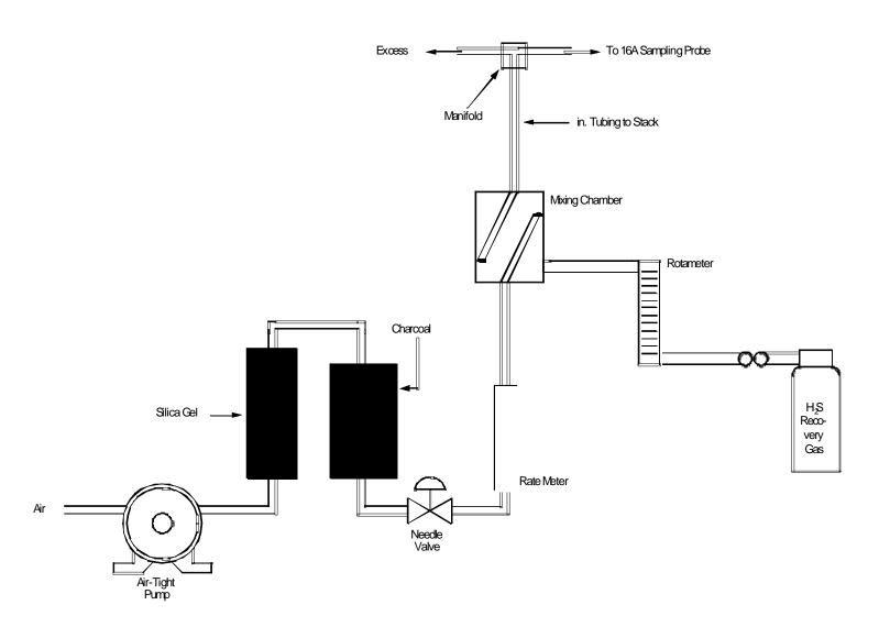
Figure 16A-3. Recovery Gas Dilution System.
