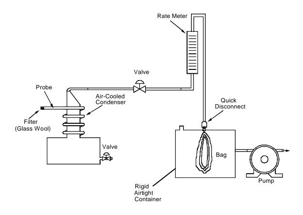
Figure 10-2 Integrated Sampling Train
