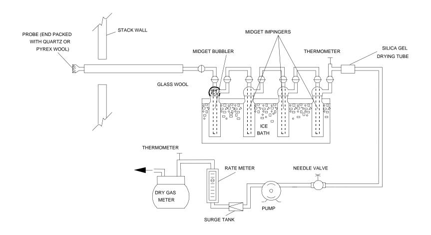
Figure 6-1. SO<sub>2</sub> Sampling Train
