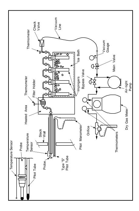
Figure 5.1 Schematic of Method 5 Sampling Train
