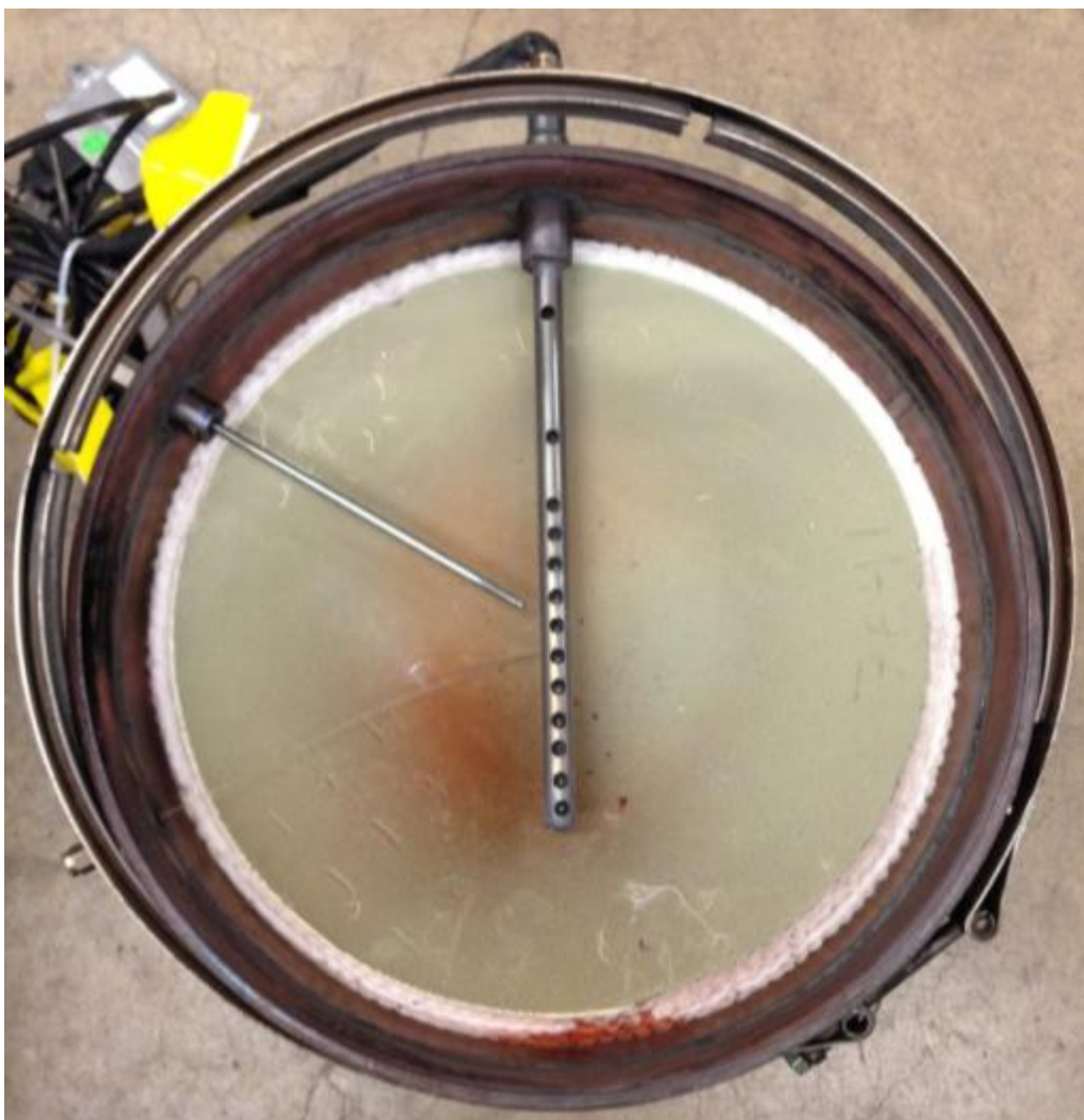
FIGURE 184. SCR CATALYST INLET SHOWING \text{NH}_3 SENSOR PROBE (AND PRODUCTION TEMPERATURE SENSOR)
