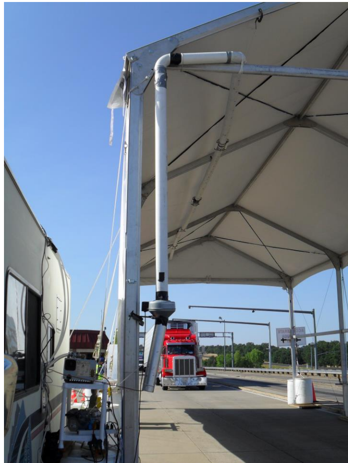
Figure 2. Photograph showing a closer view of the exhaust sampling pipe anchored to the roof of the tent. The inline fan is the metal oval between the two sections of pipe.
