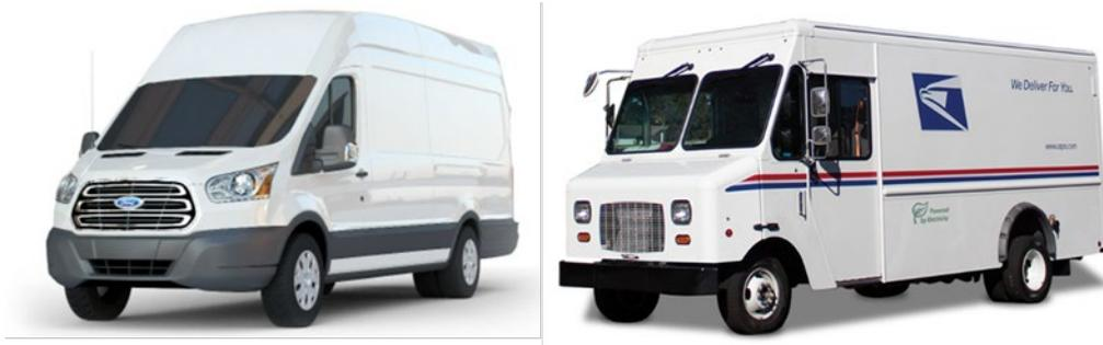
Cargo vans have a cargo area that can be accessed from the inside of the vehicle and commonly have a sliding side door and rear doors to load and unload cargo. Step vans are more rectangular in shape and are designed so the driver can easily enter the cargo area from inside the vehicle enabling frequent stops.
